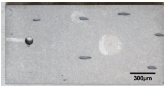
Figure 3. Light microscopy of the 125Y specimen after 1000 h in Pb-Li at 700°C.
