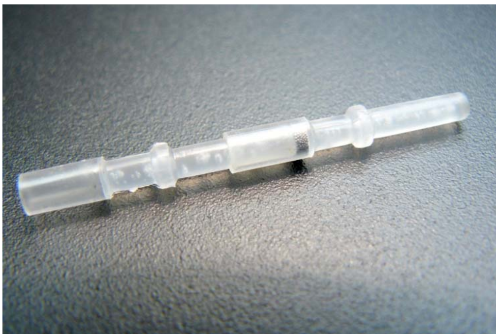
Figure 4-3. Typical mounting apparatus for a magnetization sample. Photo courtesy of Astronautics Corporation of America.
