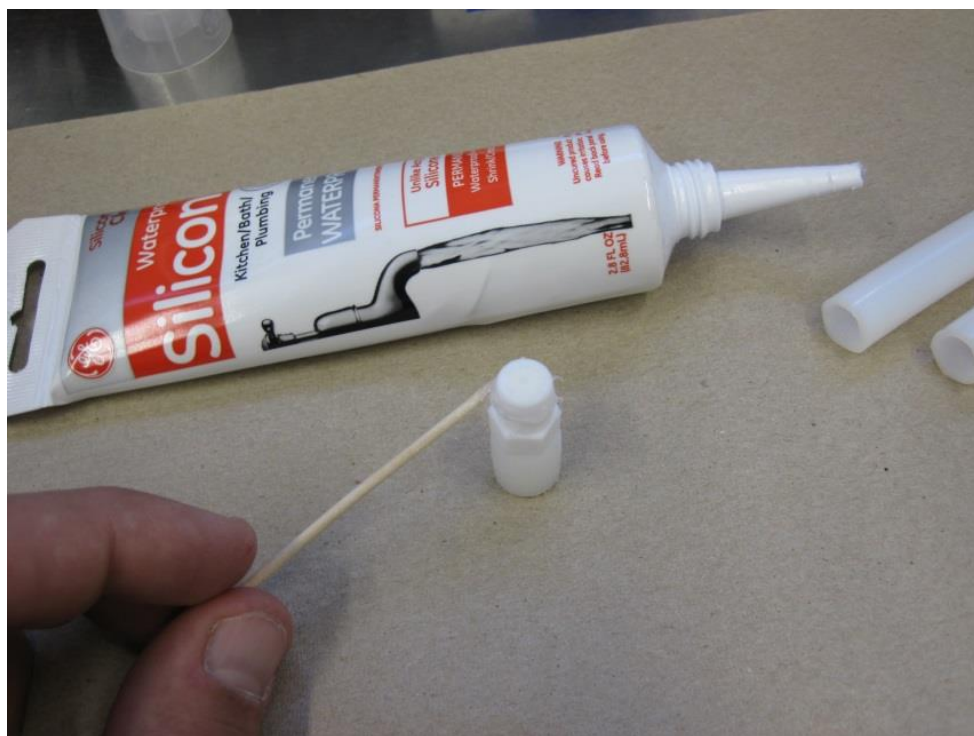
Figure 4. Image of small PEEK disk being attached to the top of a Teflon® compression fitting with silicone adhesive. and packaging for PTFE tubing (right).
