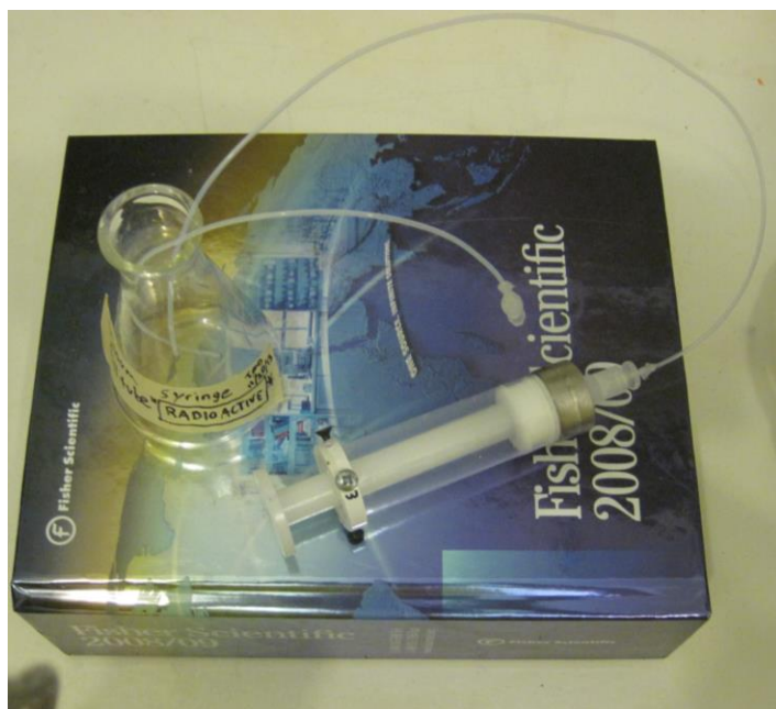
Figure 9. Modified Teflon® syringe and constructed fill tube.
