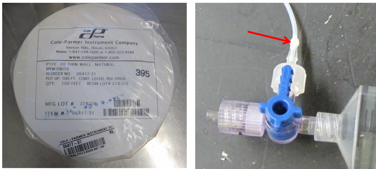
Figure 5. Epoxy seal to attach PTFE tubing inside barb end of polyethylene female Luer lock fitting.
