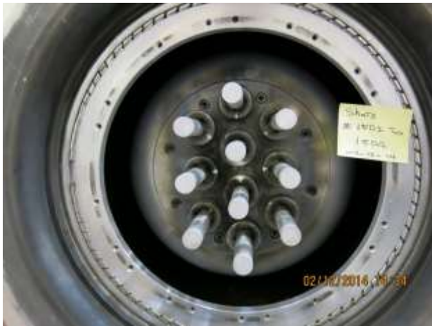
Figure 23 Anode feed plate and rods after 8 shots.
