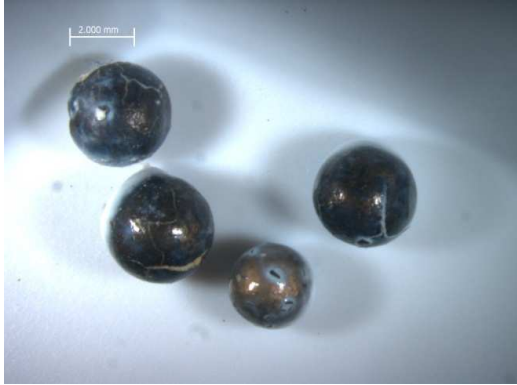
Figure 34. Optical micrographs of nickel coated PII-36 after heating to 350 °C in HiTec salt
