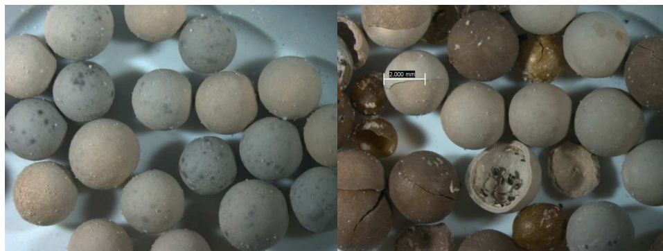
Figure 8. Images of samples PII-25 and PII-26, with 10% and 30% \text{CaCO}_3 in the shell, after heating to 350 °C.
