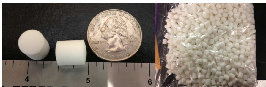
Figure 37 Potassium nitrate pellets made with tableting press.
