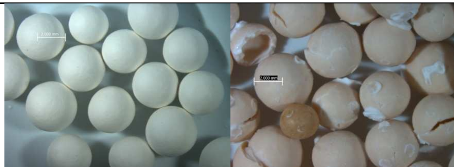
Figure 27. Sample PII-34 before and after 600 cycles in TerraDipper.
