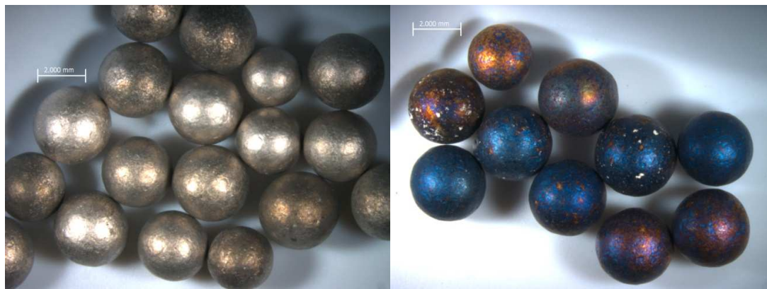
Figure 33. Optical micrographs of nickel coated PII-36 after heating to 350 °C
