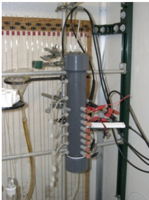
Figure 15. Column with electrodes for induced polarization measurements.
