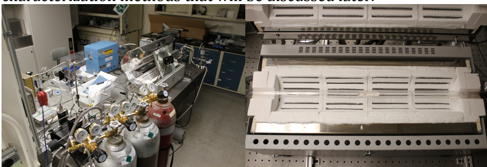
Fig. 1 (a) Cooling down the CVD with a rapid cool down. Fig. 2 Au foam in CVD before annealing.
