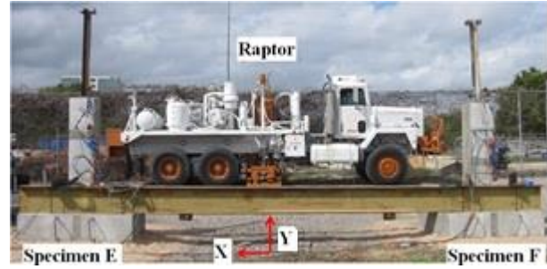
Fig. 5.46 Test setup for P wave excitation
