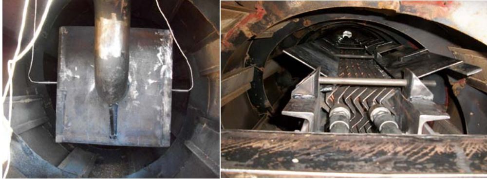
Figure 7.4 – Corrugated Plate Heat Exchanger installed with RTDs
