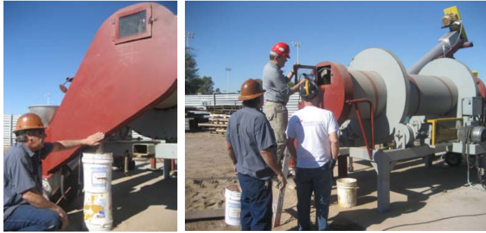
Figure 12-4: 50 kW Prototype Sand Flow Rate Experiments
