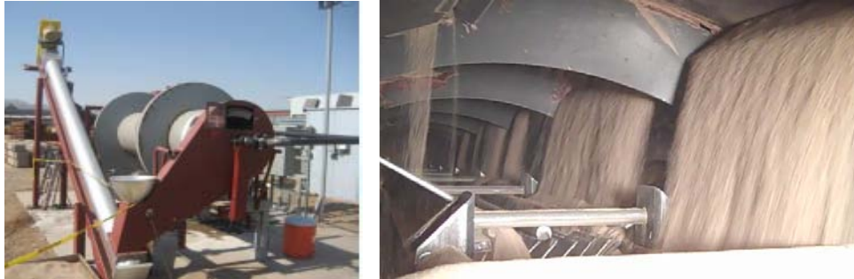
Figure 7.2 – 50 kW Integrated Prototype System (testing of corrugated plate heat exchanger shown on right)
