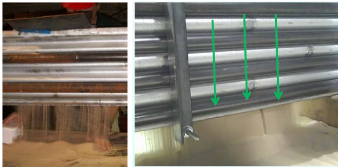
Figure 12-5: Sand Flow Through the Corrugated Plate Heat Exchanger
