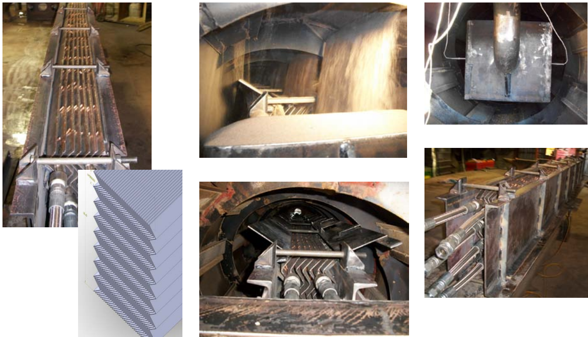
Zig Zig Tube bundle Design Concept and as Fabricated for 50 kW unit
