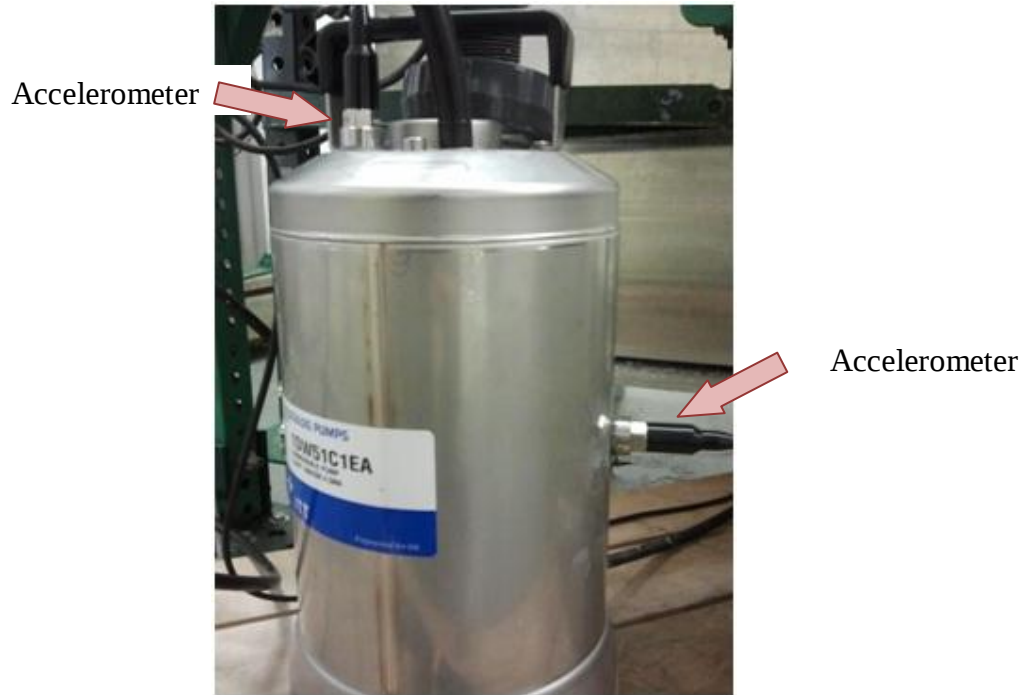
Figure 3.12: Positioning of the two accelerometers on the pump casing
