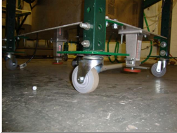
Figure 3.4: Water tank support structure with wheels and adjustable brakes
