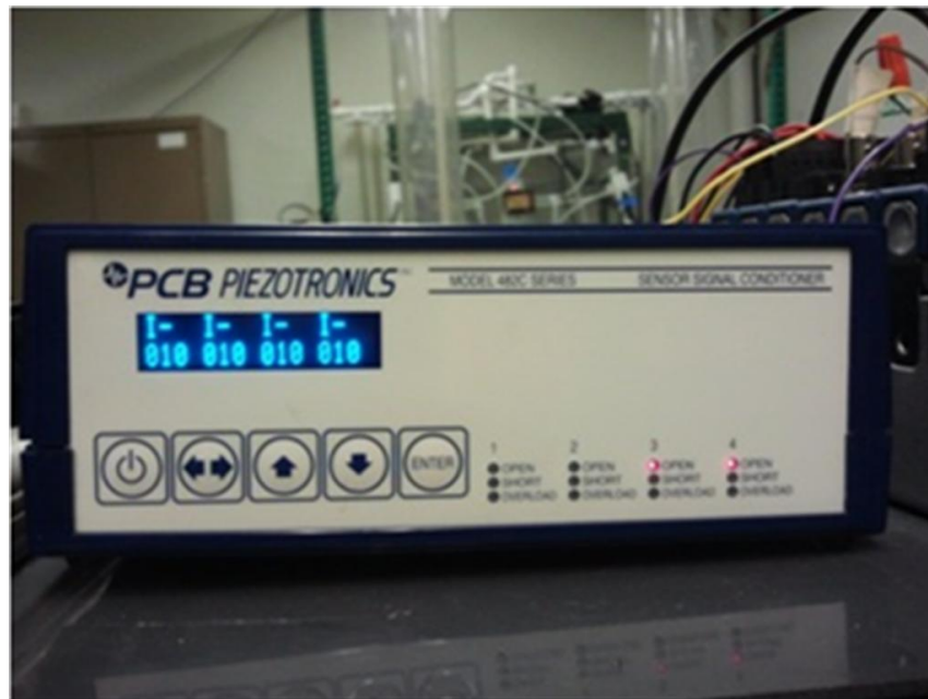
Figure 3.11: Signal conditioner used with PCB accelerometers.
