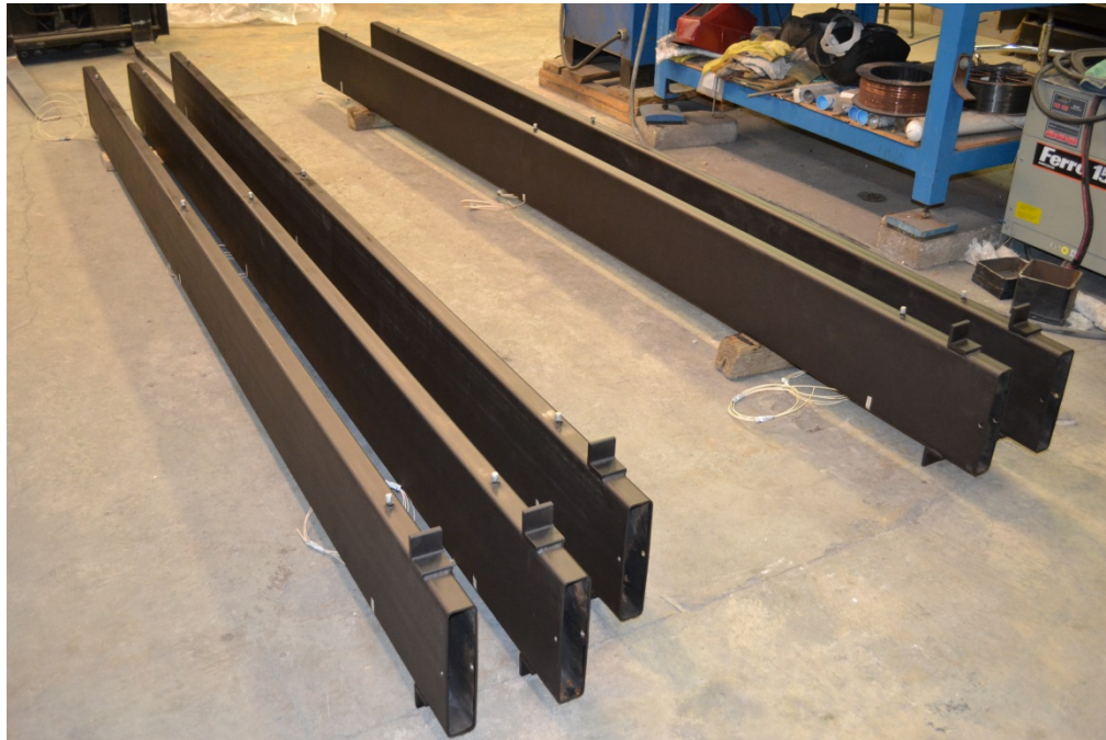
Figure 107 – Finished riser ducts (Riser 4 missing in photo).
