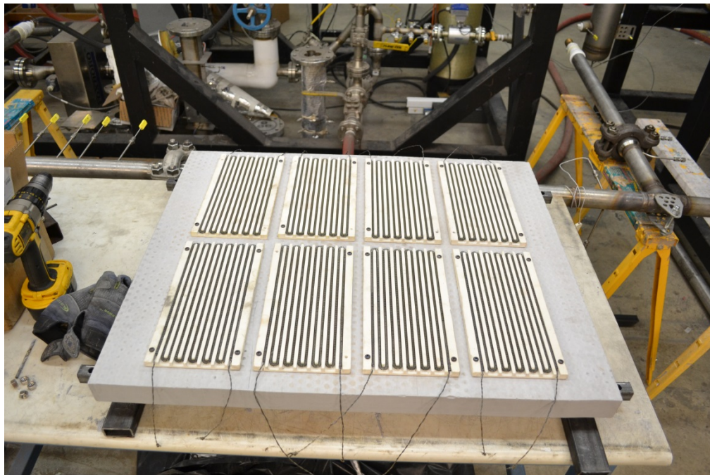
Figure 104 – Assembled heater module.
