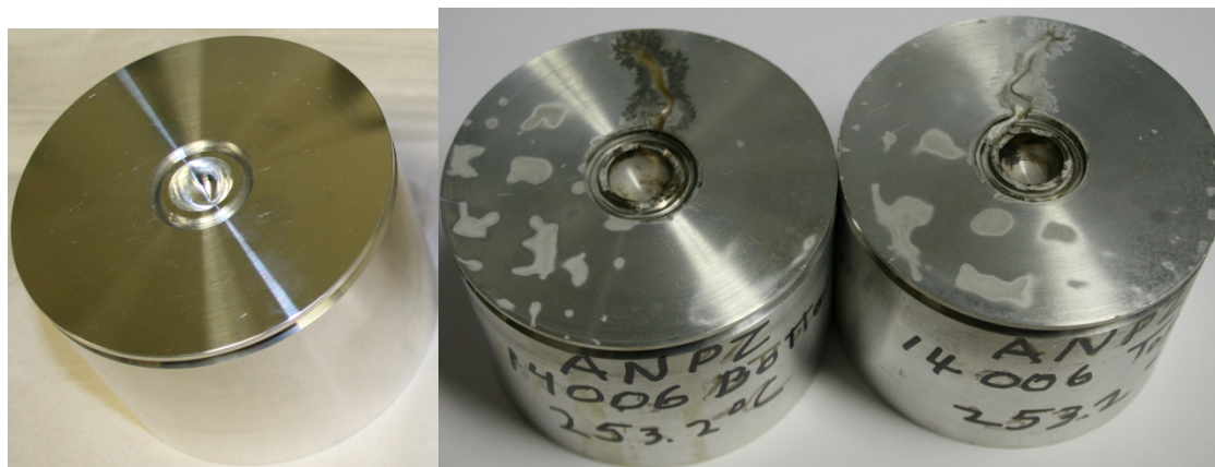
Figure 5. Anvils before and after thermal explosion of ANPZ at 253.2 C; left was the pristine anvil; also shown are bottom anvil (middle) and top anvil (right) after the thermal explosion.
