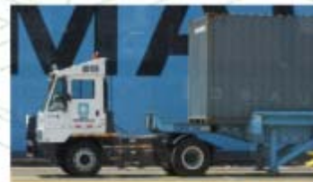
A typical yard hostler vehicle used to move containers at a sea port berth.
