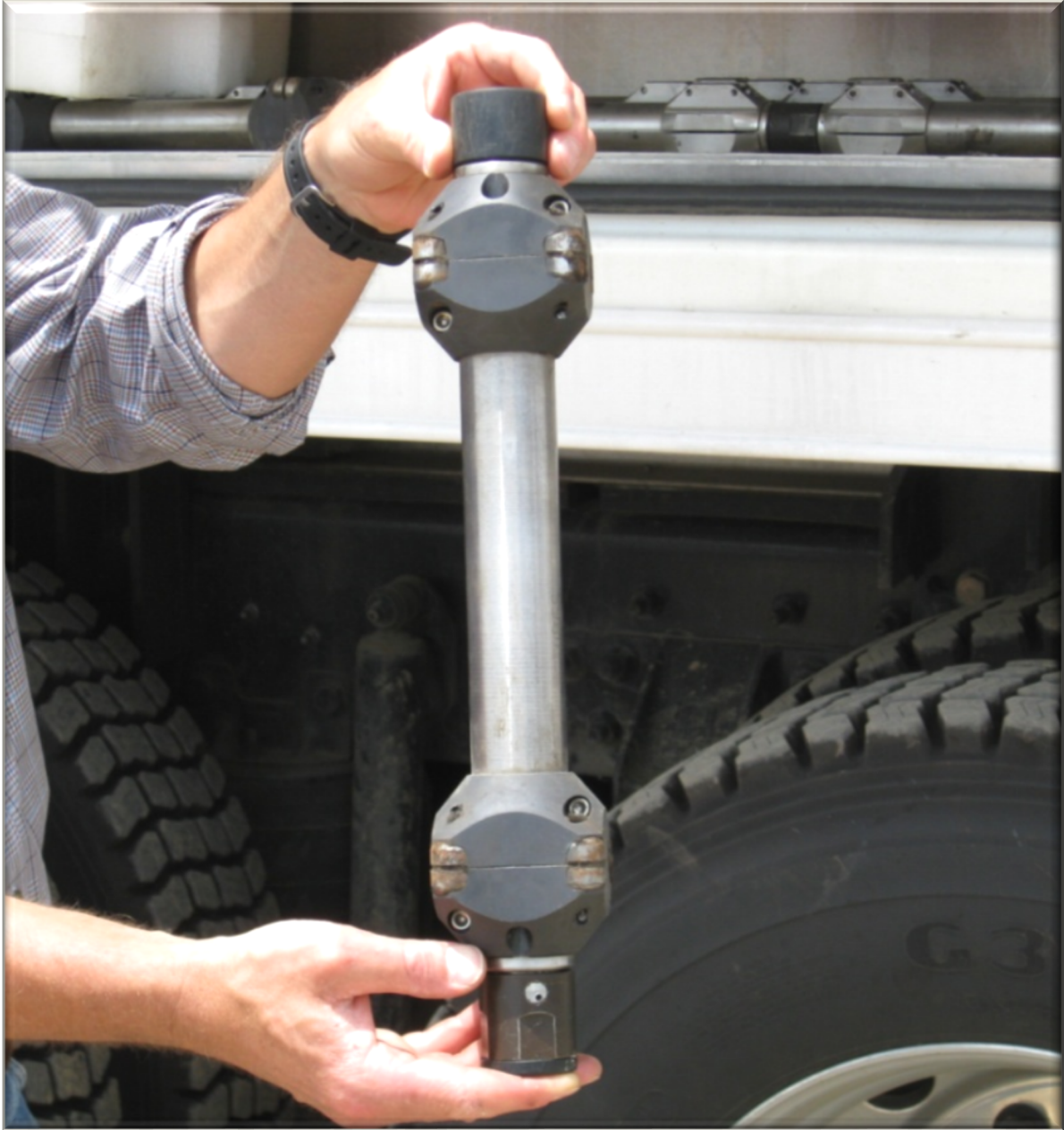
Figure 45: One of the high-grade digital geophones, manufactured by GeoSpace of Houston, Texas, deployed by the APEX HiPoint/ Sigma3 field team in the monitoring wells.
