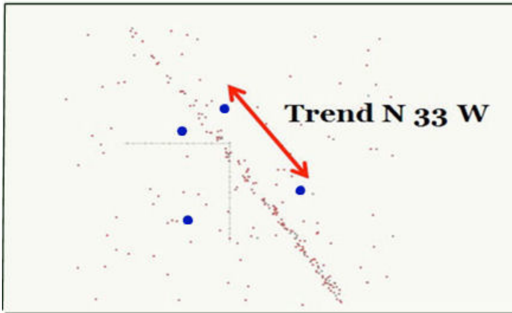
Figure 47: Southern array shows a dominant trend of episodic microseismic signals observed in the processed data. The four larger blue dots identify the four monitoring hole locations. The smaller dots represent resolved signals. The grid spacing is 100 m (Slide 27, APEX HiPoint/ Sigma 3 Southern Array Final Report to Davenport).
