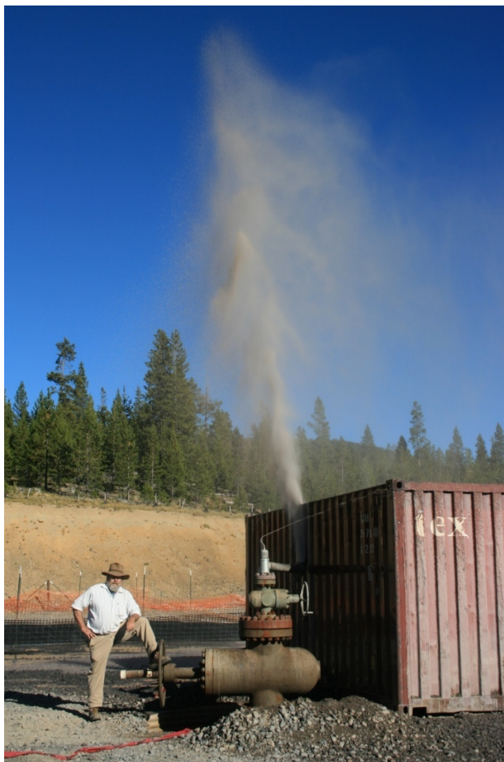
Figure 10: Drilling fluid flowing from the well NWG 46-16, approximately 45 minutes after the liquid flow commenced. (8 September 2013).
