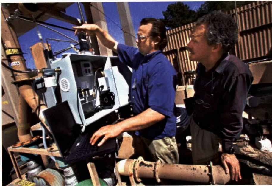
Stack air sampler calibration with oversight by staff of DOE's Berkeley Site Office
