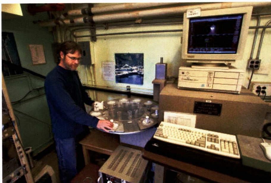
Loading environmental samples on a gamma spectrometer in Building 76
