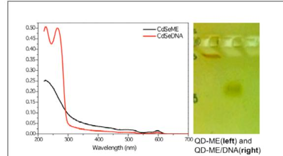
**Figure 5.** UV Vis spectra of mercaptoethanol (ME) (black) and ME+DNA (red) conjugated nanoparticles. Strong UV band at 260nm in the ME+DNA curve indicates DNA is successfully conjugated to the ME bound NPs. (Right) Gel electrophoresis showing different mobilities for ME vs ME+DNA QDs.
