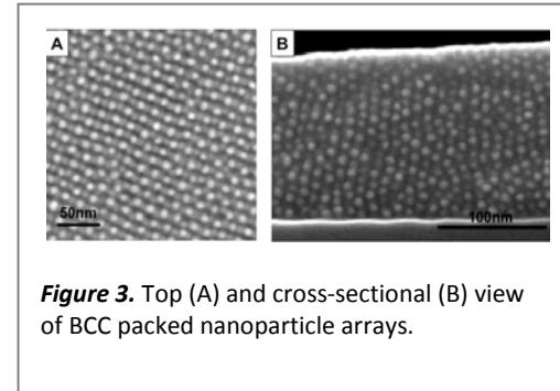
**Figure 3.** Top (A) and cross-sectional (B) view of BCC packed nanoparticle arrays.
