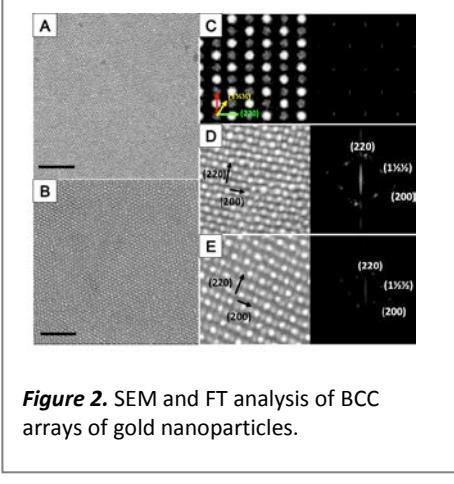
**Figure 2.** SEM and FT analysis of BCC arrays of gold nanoparticles.
