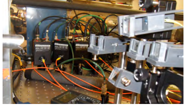
Photos of 3-channel and 5-channel configurations of the FSI test system (arrows on left indicate paths of launched and returned laser beams)
