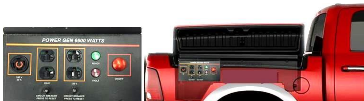
Figure 25: Auxiliary power panel vehicle integration
