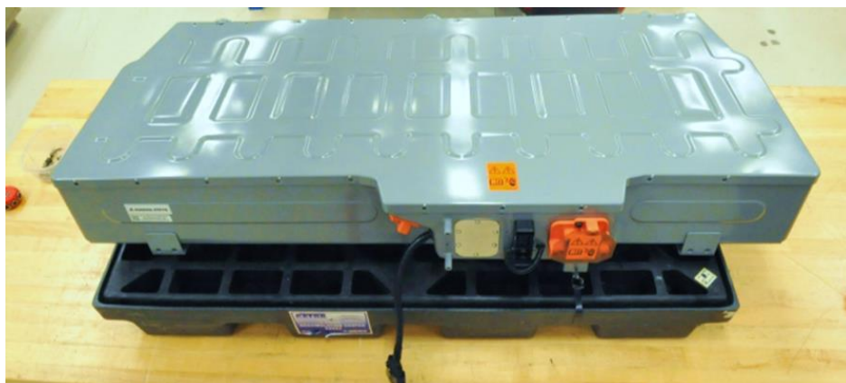
Figure 6: Magna/JCI high-voltage energy storage system as installed in Phase II
