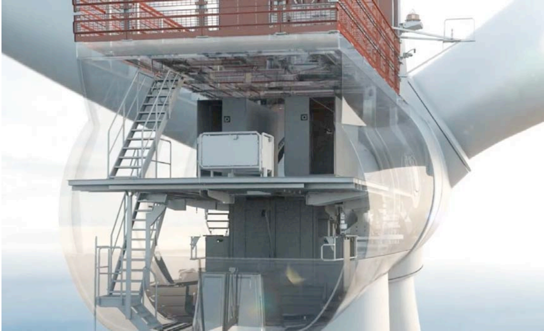
Figure 1.23 Image from a semi-transparent model of the Siemens 6 MW 154 m wind turbine nacelle, showing the yaw drives, interior electrical cabinets, and the helicopter deck.
