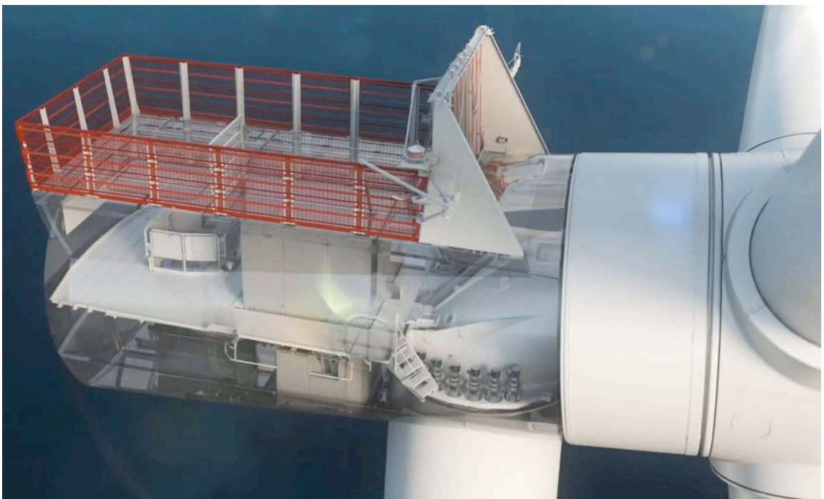
Figure 1.22 Images from a semi-transparent model of the Siemens 6 MW 154 m wind turbine nacelle, showing the yaw drives, interior electrical cabinets, and the helicopter deck.
