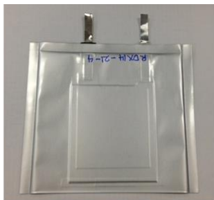
R&D Cell Capacity: < 100 mAh Size: 95 x 95 x 0.4 mm
