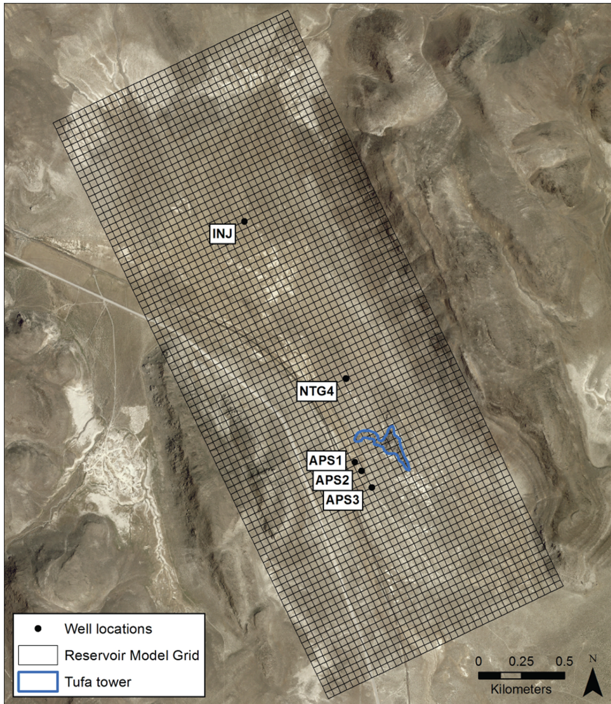
Figure 11. Astor Pass geothermal model grid showing locations of APS-1, APS-2, APS-3, NTG4, and theoretical injection well used in the exploitation scenarios for energy scaling.
