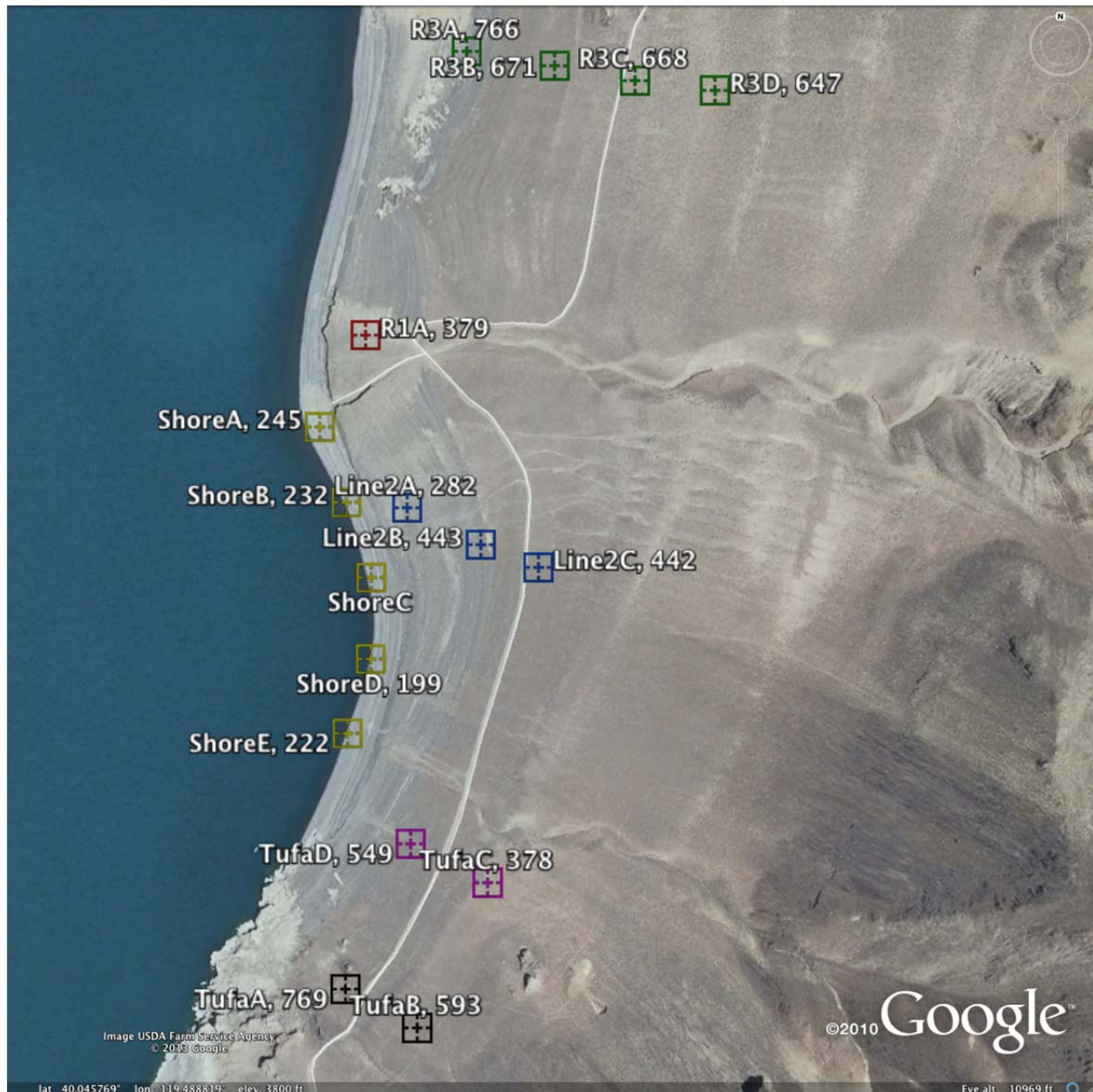
Figure 40. The locations of the refraction microtremor results tagged with their individual array name and Vs30 values (m/s). From Google Earth Pro.
