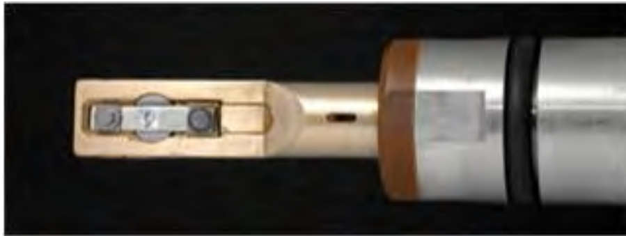
Figure 3.8: An in-situ TEM deformation holder with a sample loaded
