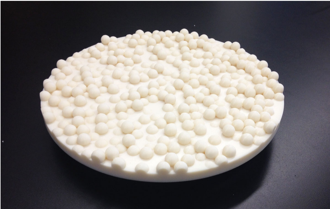
Figure 2-39. Random packing piston plate for use in the Cylindrical Silo test section.
