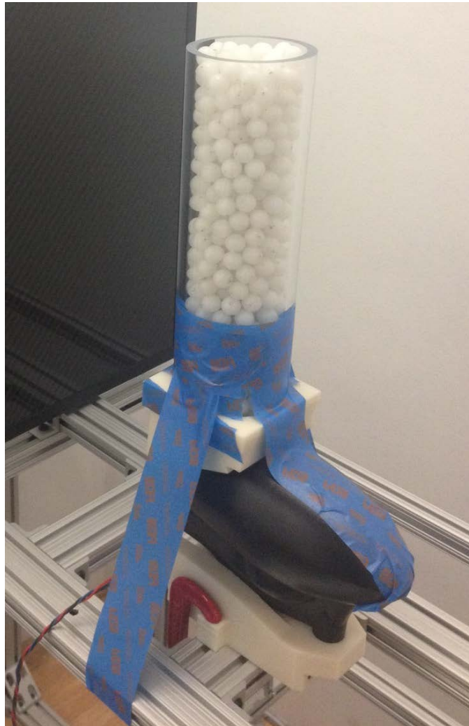
Figure 1-50. Continuous discharge device set up for testing and verification of the X-PREX image processing modules. The upper section within the x-ray imaging area contains 470 pebbles.
