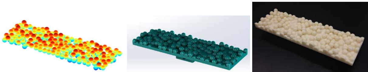
Figure 2-7. Random packing configuration from DEM simulation (left), CAD model (center), and FDM-manufactured random pebble packing piston plate (right).
