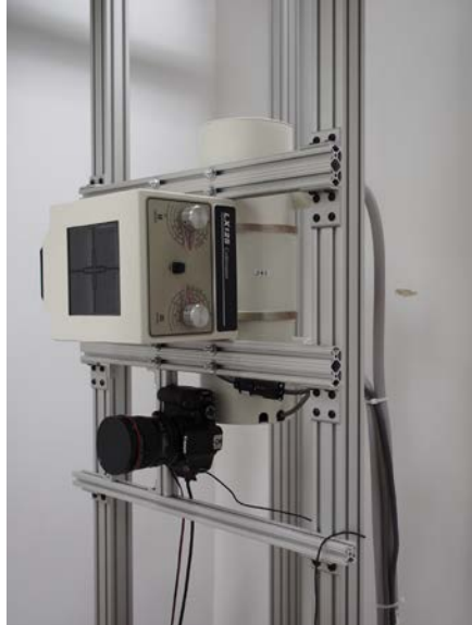
Figure 1-6. View of the x-ray tube and the remote visual camera mounted in line with the focal point.
