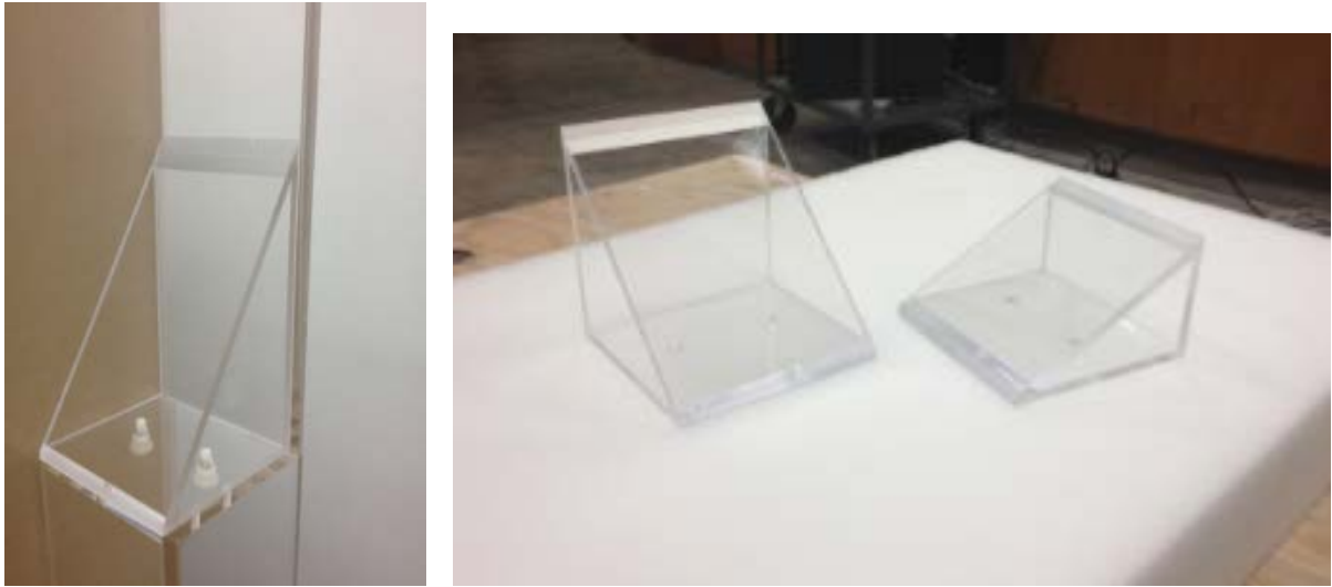
Figure 2-3. Detail views of the 60-degree wedge installed on the test section (left) and the 45 and 30-degree wedges (right).
