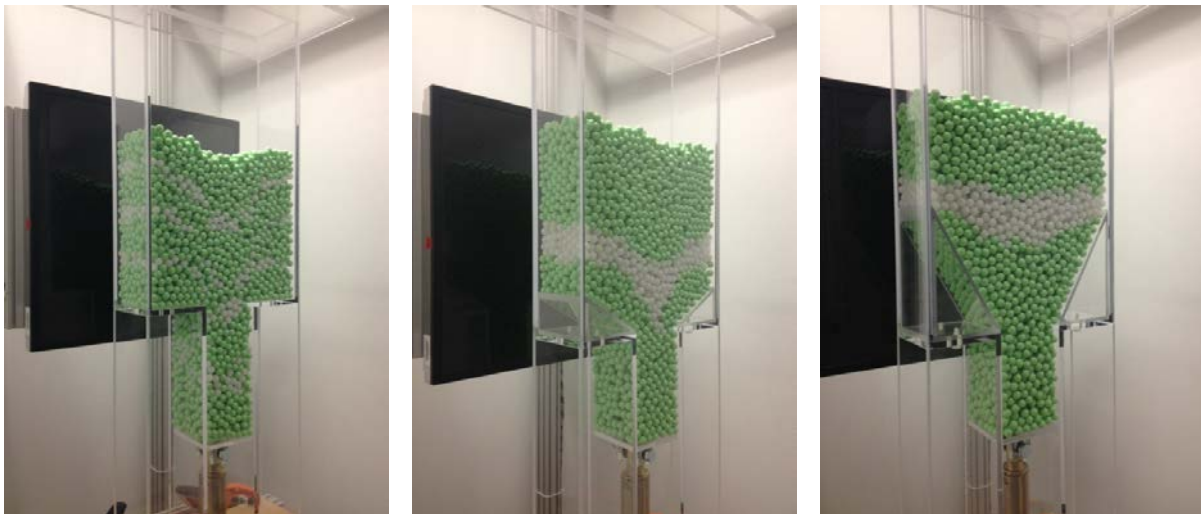
Figure 2-4. Images of the Quasi-2D Silo Test Section in the modular test bay during data collection for the 0-degree (left), 30-degree (center), and 60-degree (right) converging configurations. The white pebbles in the images are instrumented with tungsten wires, while the green pebbles are unmodified HDPE pebbles.
