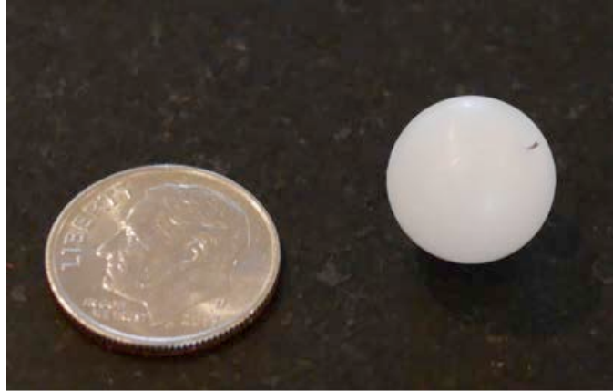
Figure 1-28. Detail view of a single instrumented pebble. The small end of the tungsten wire can be seen at the upper right side of the pebble. The wire ends are finished with a grind wheel to ensure a smooth pebble surface.
