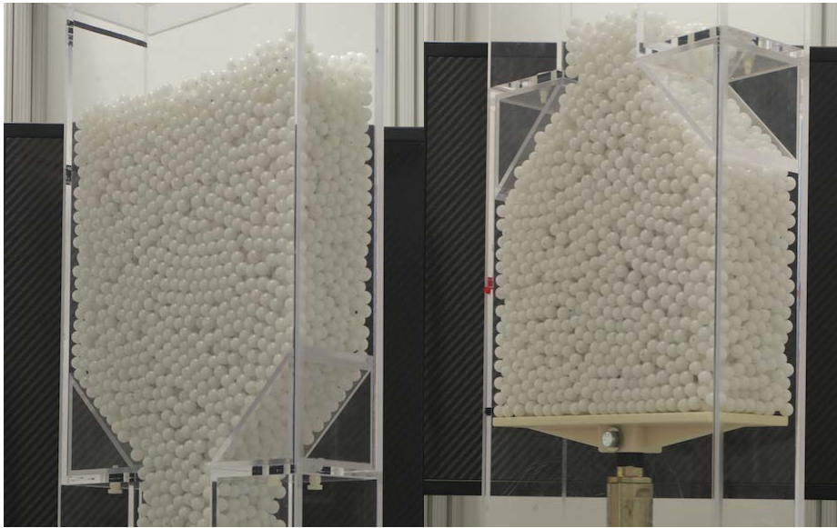
Figure 2-5. Converging (left) and diverging (right) configurations of the Quasi-2D Silo test section with a 45-degree hopper angle.
