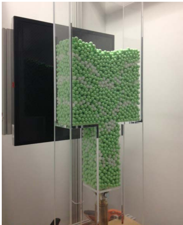
Figure 2-1. Quasi-2D Silo test section in the X-PREX facility. For the test show here, 3,000 pebbles were initially loaded into the test section then downward motion of the pebbles occurs as a piston plate in the orifice chute moves in incremental steps of d .
