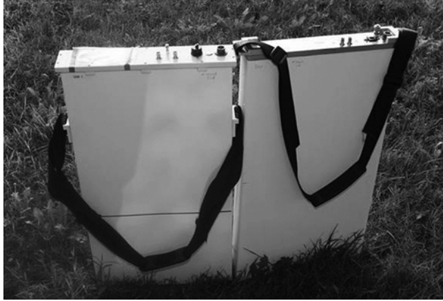
Fig. 4. Two-panel NMC. The left panel has 100 straws and the right one has 60 straws. Each panel's external dimension is 70 \times 40 \times 6.25 cm and the combined weight is 29.4 kg (64.8 lb).
