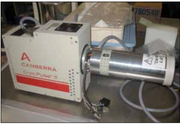
Figure 120.119 Germanium detector with its electronic cryogenic module.
