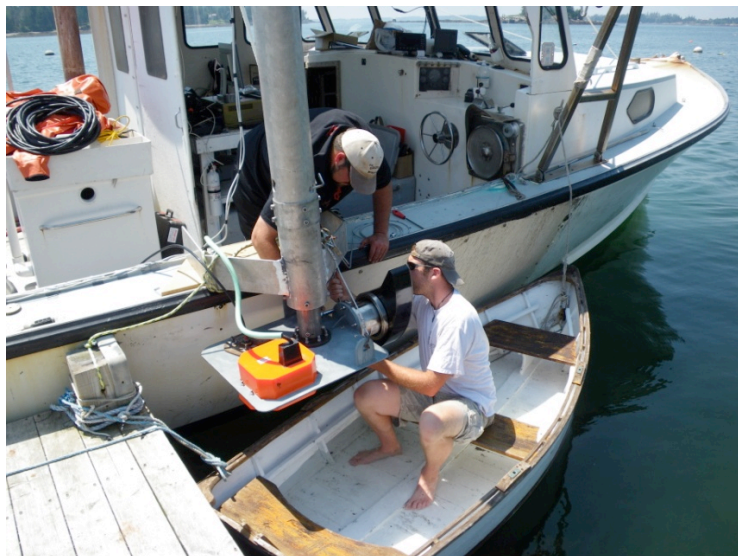
Figure 3. Mounting of acoustic equipment to survey vessel – F/V Seldom Seen
