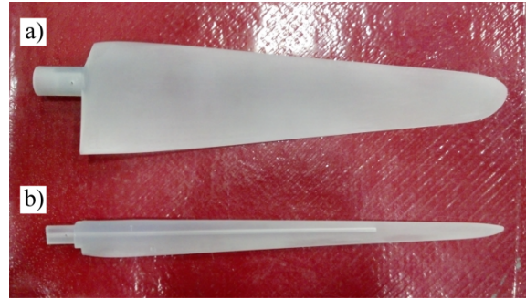
Figure 128: Images of a) redesigned, thrust-matched blade and b) original geometrically-scaled, NREL 5 MW reference wind turbine blade.
