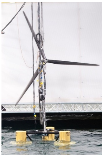
Figure 2: 1/50 th scale model NREL 5 MW Reference Wind Turbine mounted to a semi-submersible platform.
