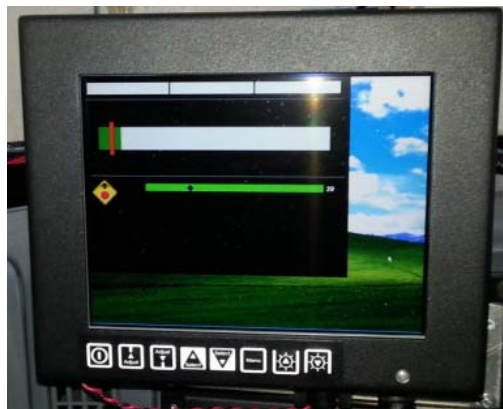
Figure 20: VGA based, 7in display for HMI simulator study
