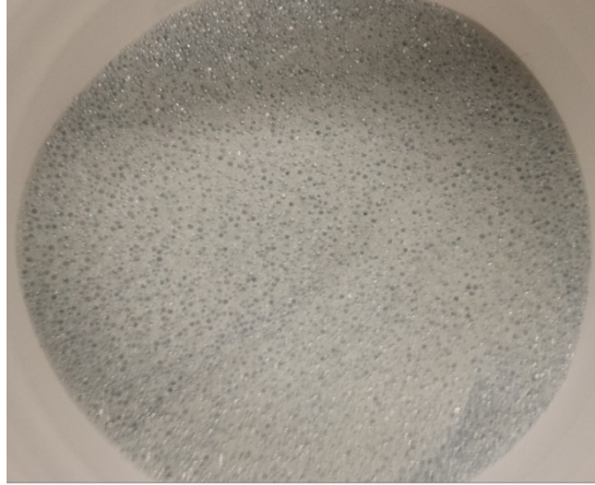
Figure 167: Mechanically and evenly mixed beads of 0.5mm (50%), 2mm (25%), 3mm (25%) to form the store with local heterogeneity.
