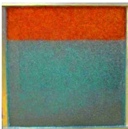
Figure 123: Initial condition of the closed-state experiment. After packing granular medium of hydrophilic beads in the apparatus, aqueous phase (blue) (the brine/glycerol mixture) was slowly injected from the bottom to fill entire medium, followed by slow injection of light mineral oil/decane mixture (red) from the top to displace aqueous phase through the bottom. To initiate the buoyancy driven displacement, the gravity-stable configuration shown in this photograph is reversed by pivoting the apparatus 180 degrees in the frame (a rotation around a horizontal axis through the middle of the domain in the photograph), thus the denser aqueous phase is placed above the less dense hydrocarbon phase.
