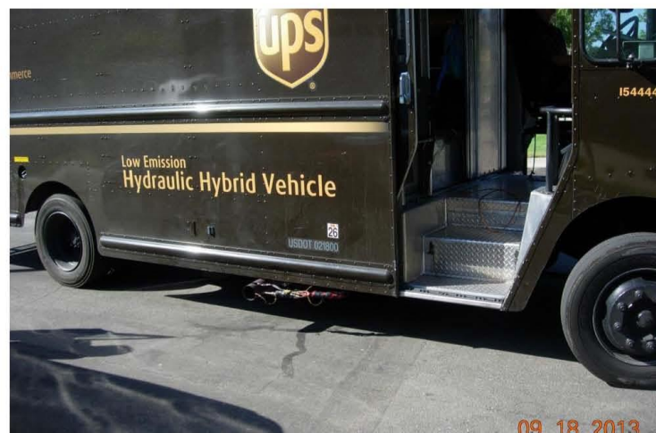
Figure 4: Isokinetic probe and sample line installed in the exhaust outlet of the hybrid vehicle
