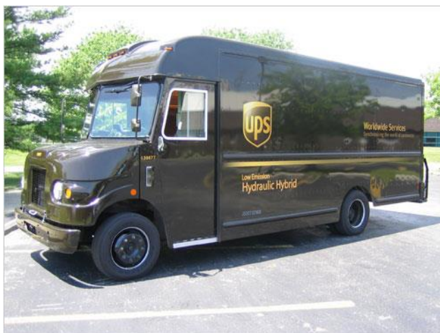
Figure 5: The U.S. EPA / Eaton hydraulic hybrid parcel delivery truck (left) and the description of the Eaton series hydraulic hybrid system [9]
