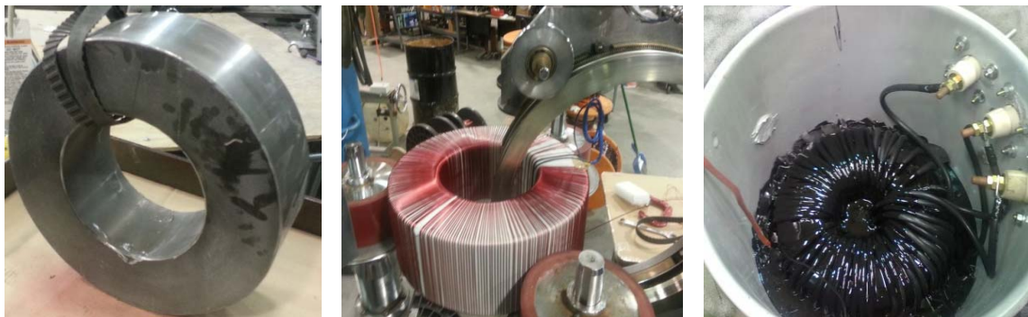
Figure 1.2. Arrangement of core and windings (active element) of the new toroidal distribution transformers.
