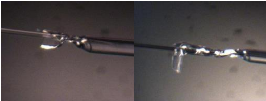
Figure 5-12: CO 2 laser bonding around the porous tube with applying laser more than 10 times
