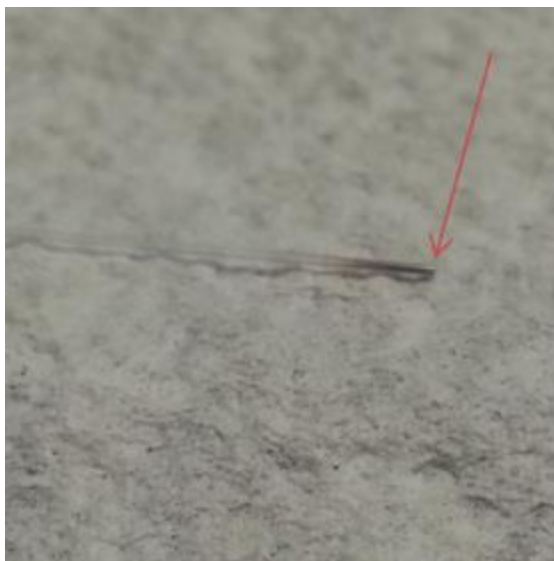
Figure 5-58: End of capillary tube clogged with plating solution.
