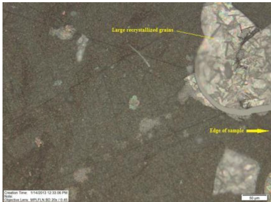
Figure 4-16: Bond interface of colloidal alumina fired in the presence of chromium suggests some recrystallization occurs
