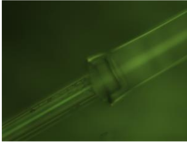
Figure 4-169: Splicing between MM and Sapphire fiber with GRID MM fiber
