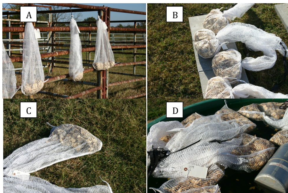
Figure 3. Wood chip samples exposed to their assigned treatments: (a) air, (b) paved, (c) soil, and (d) water.
