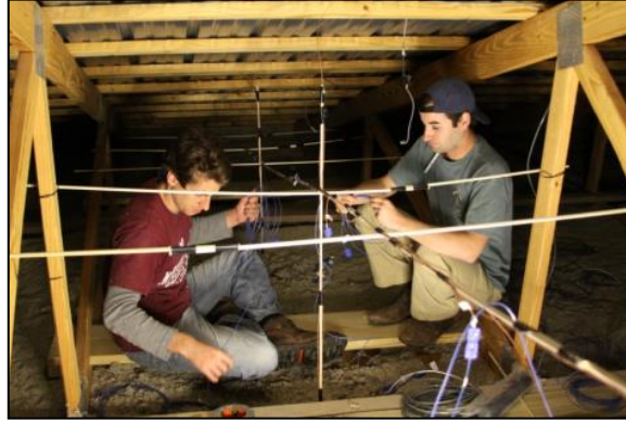
Figure 3: Graduate students installing thermocouples on the cross-sectional array made with dowels.
