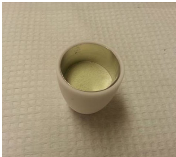
Figure 1. Reaction vessel consisting of a platinum crucible inserted into a ceramic crucible containing powdered reactants
