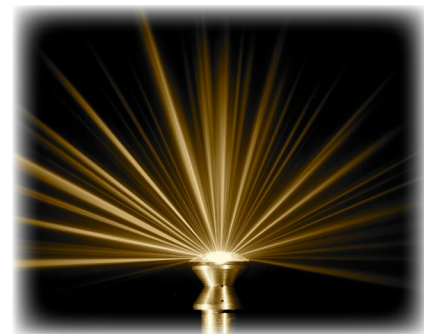
An advanced optical probe used with multiplexed photonic Doppler velocimetry (MPDV) for dynamic material experiments
