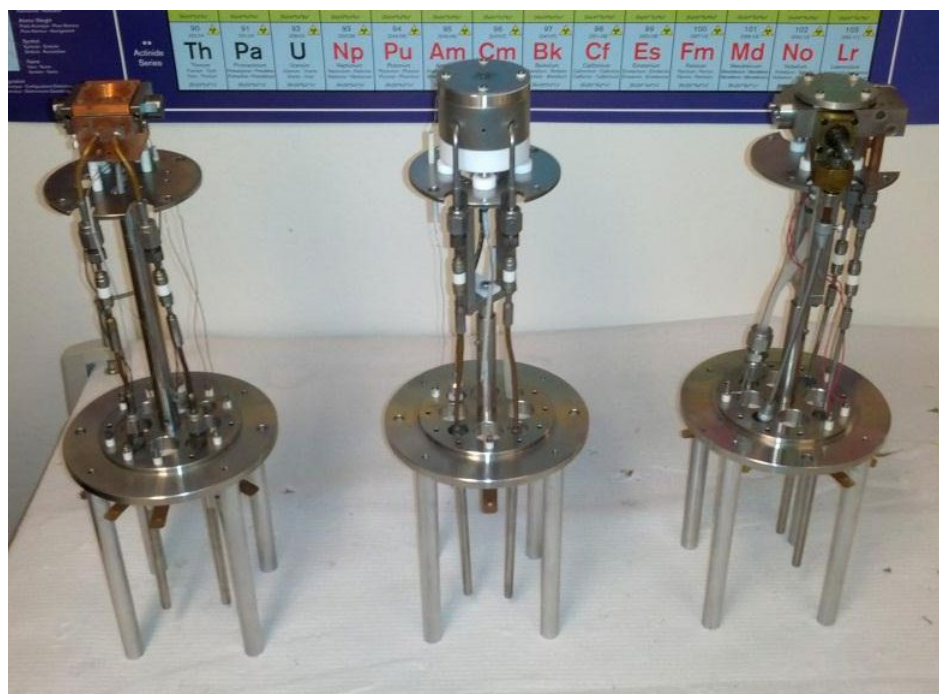
Figure 3. The three ionization sources developed for use with the instrument. The sources shown (left to right) are an electronic impact source, a DC-discharge source, and a laser vaporization source.
