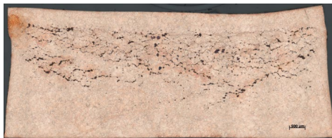
Figure 16. Optical image of the cross-sectioned 4.18 mm NM-driven copper sample (Shot 9). The regions of shear localization linking voids along 45^\circ to the sample outer diameter are consistent with late time, radial release-induced damage evolution.
