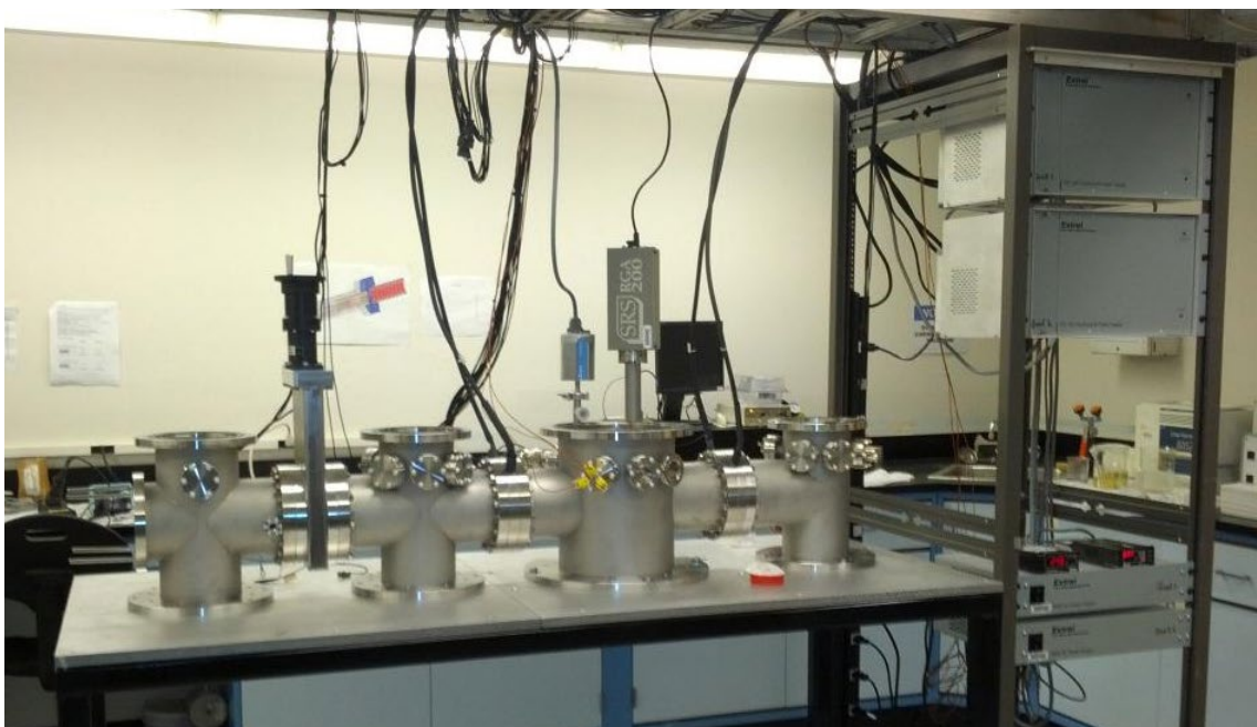
Figure 2. The assembled quadrupole-cell-quadrupole instrument. The chambers shown (left to right) are the ion source chamber, the first quadrupole chamber, the main chamber, and the second quadrupole/detector chamber. The various subassemblies are housed within these vacuum chambers.
