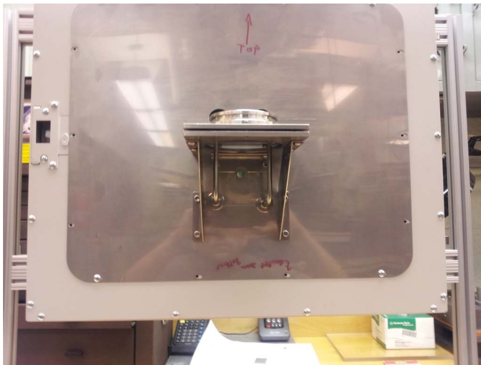
Modified door for the 300 °C EDB showing electrical and gas feedthroughs.
