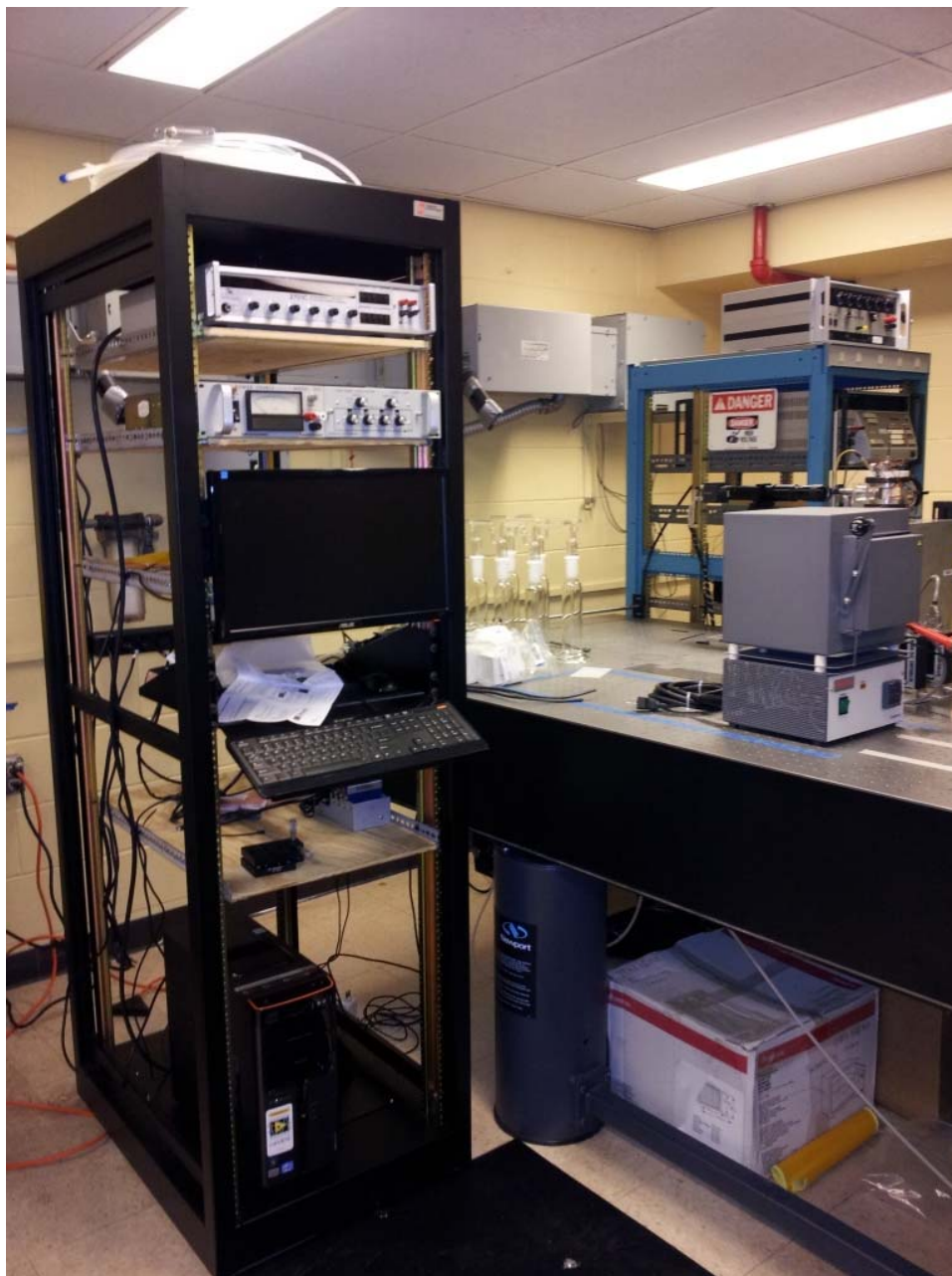
Data acquisition and levitation electronics for the very high temperature EDB. The high temperature furnace in 'as received' condition is shown at right before the door was removed and EDB modifications were made.
