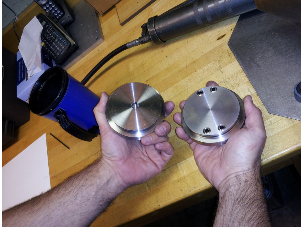
Haynes 230 top and bottom end caps for low-temperature EDB.
