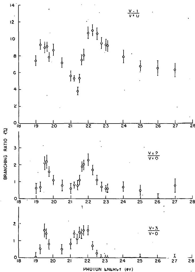
FIG. 1.--Photoionization branching ratios for the  $v = 0-3$  levels of  $\text{CO}^+ \text{X}^2\Sigma^+$ .
