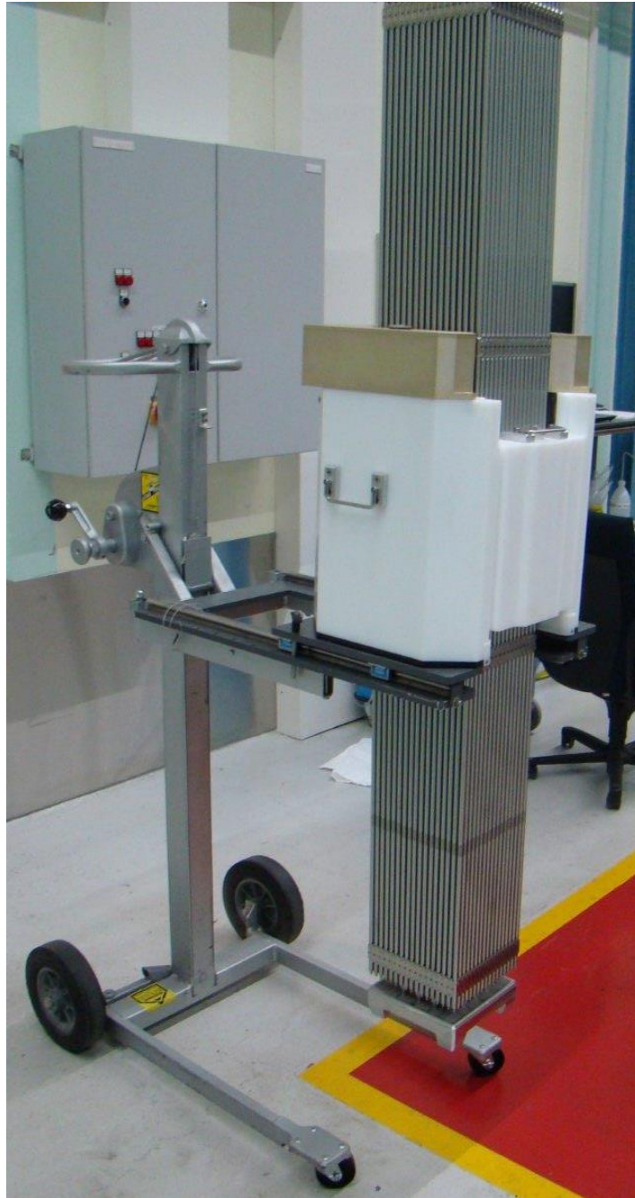
Figure 3 EFC Mounted on Cart with Fresh Fuel Assembly in Measurement Position
