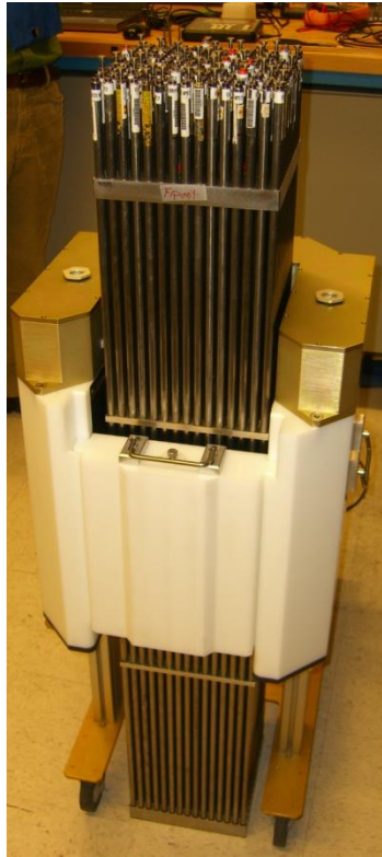
Figure 2 EFC during measurement of Fuel Assembly Mock-up
