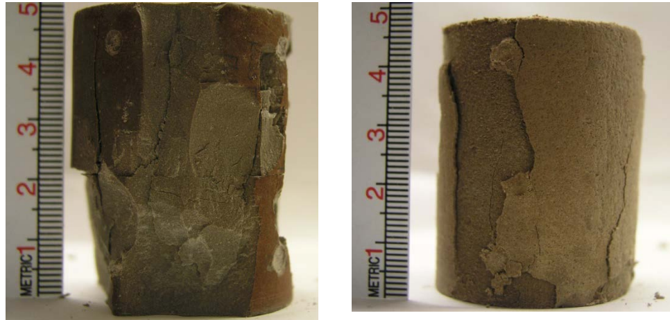
Figure 5. One to three week alteration images. The alteration photos for 1 and 3 week samples are treated with phenolphthalein.
