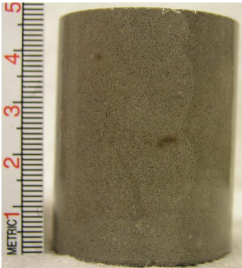
Figure 11. NM2_5 \mu m_27.5%_MINUSIL 40%. (A) initial core. (B) Core cured 1 week in Ormat/CO 2 brine. Sample treated with phenolphthalein.
