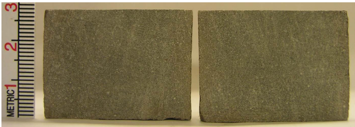
Figure 7. Fmix1, 3 week cure in Ormat brine/CO 2 . Right sample is treated with phenolphthalein. No color change indicates pH < 10.
