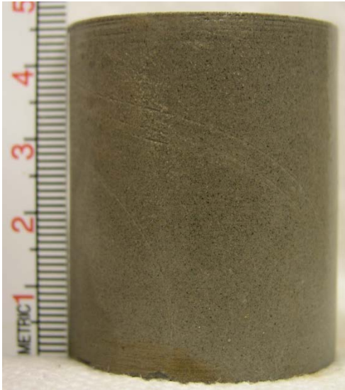
Figure 10. NM2_5 \mu m_27.5%_MINUSIL 20%. (A) initial core. (B) Core cured 1 week in Ormat/CO 2 brine. Sample treated with phenolphthalein.
