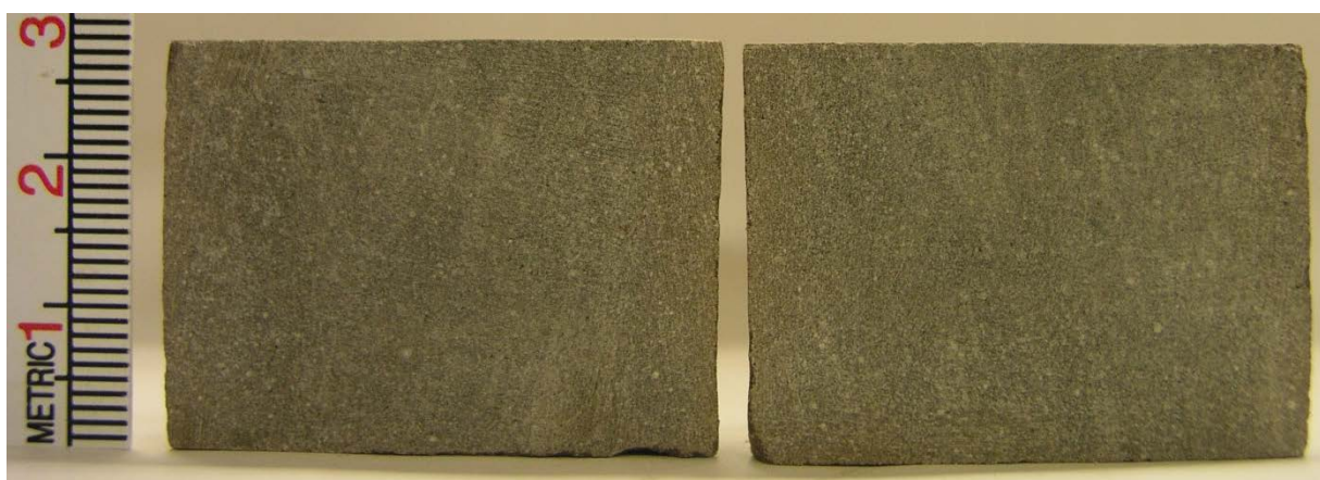
Figure 2. Fmix1, 3 week cure in Ormat brine/CO 2 . Right sample is treated with phenolphthalein. No color change indicates pH < 10.
