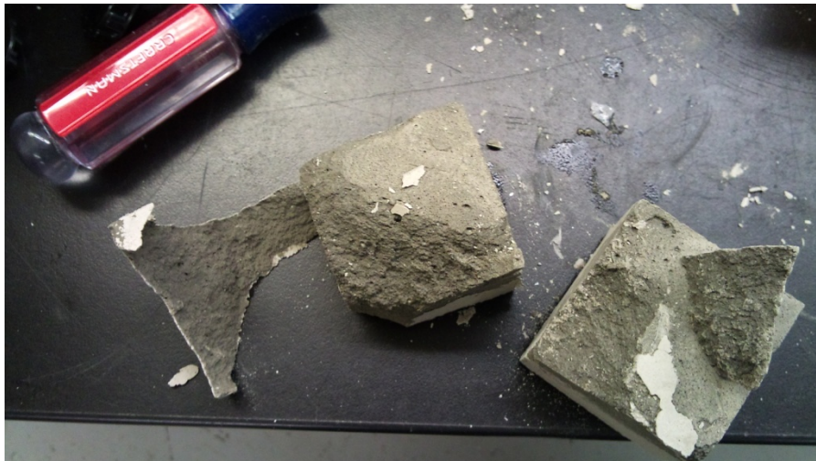
Figure 12 Damaged Ferrierite samples while de-molding
