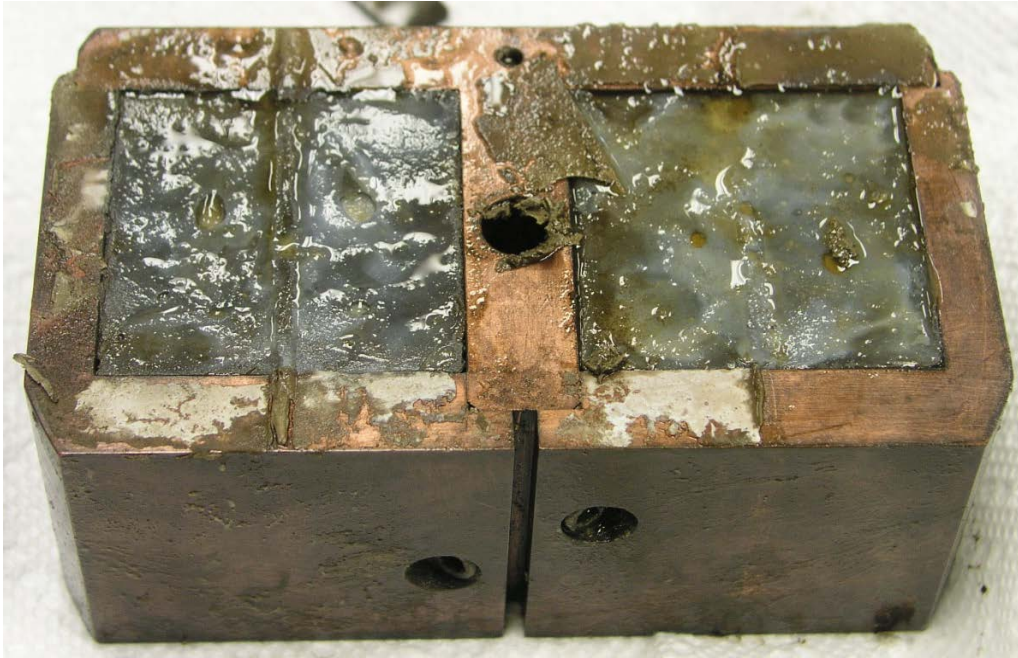
Figure 4. Image of typical Fmix1 molds showing potential free water.
