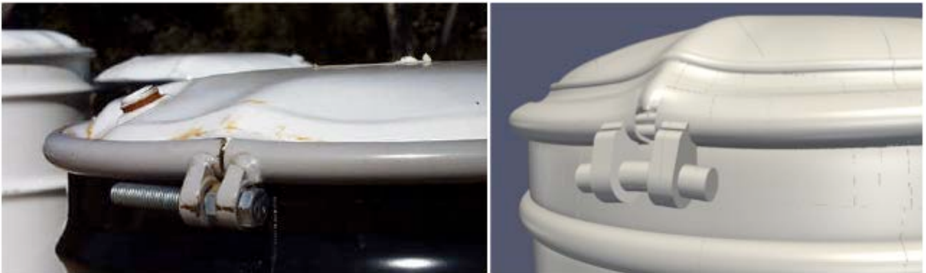
Figure 8. Comparison of tested drum at LANL (Larranaga et al., 1999) left, and analysis results, right.
