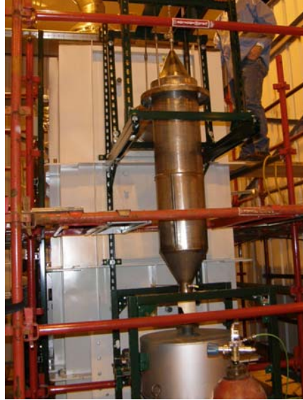
Figure 70 – Ejector, Prereformer, Circulator
