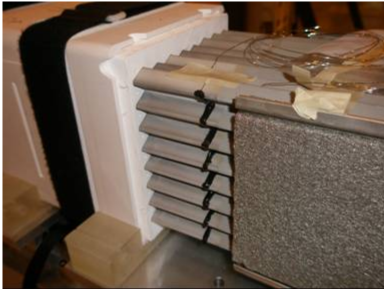
Figure 53 – Bundle Assembly Showing Open-end Seal, Casting and Instrumentation
