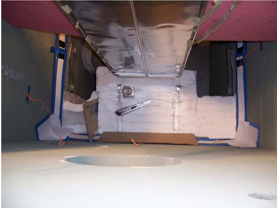
Figure 22 - Exhaust Manifold on Bottom of Container
