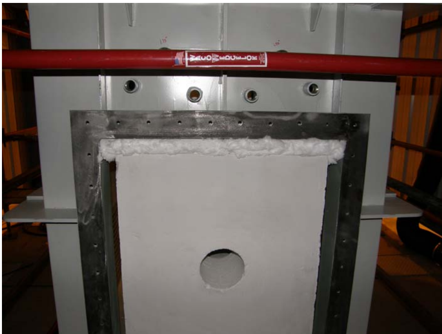
Figure 23 - Exhaust Manifold and Outlet Insulation Packing
