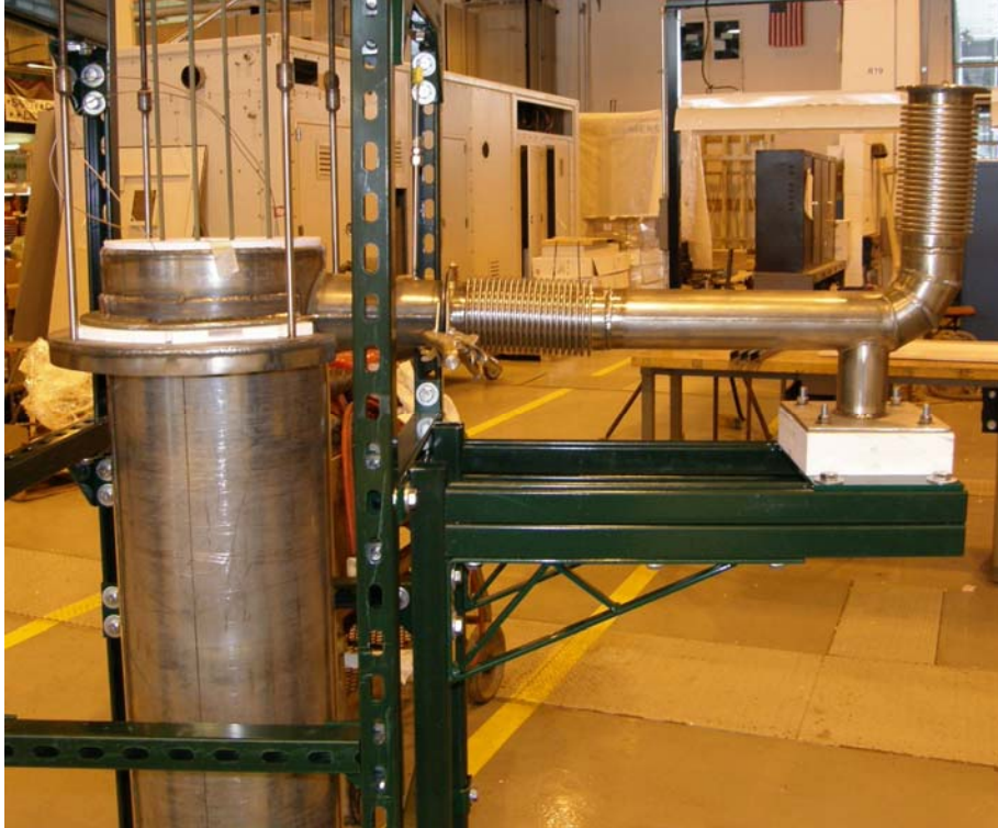
Figure 29 – Heater No. 1 and Recirculation Loop Pipe Spool
