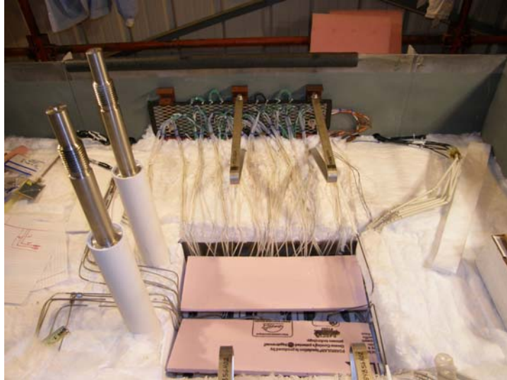
Figure 62 – Instrumentation from Stack to Container Wall
