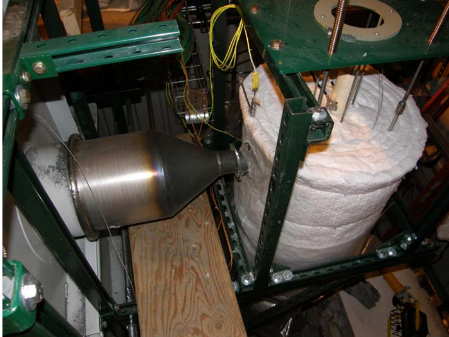
Figure 33 – Fuel Heater No. 2 and Container Inlet Feed-through with Insulation Removed (post-test)
