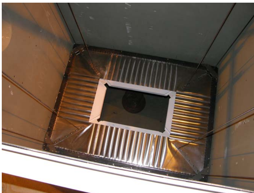
Figure 8 - Fuel Barrier in the Installed Position
