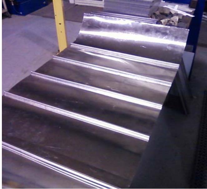
Figure 5 - Liner Test Bends to Verify Pleat Spacing
