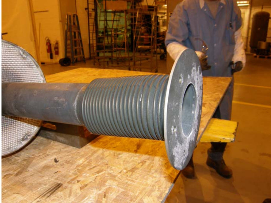
Figure 35 – Feed-through Bellows (post-test)
