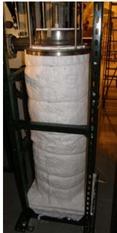
Figure 73 – Insulated Lower Fuel Heater
