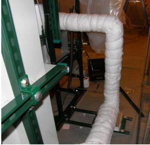
Figure 72 – External Loop Piping Insulation
