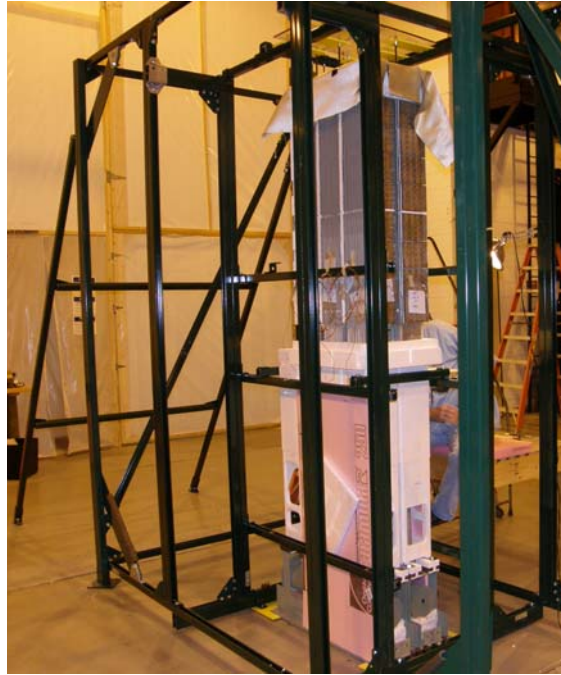
Figure 54 - Placement of Bundle Rows onto the Stack Tray
