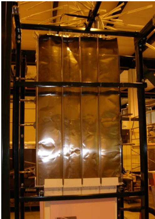
Figure 6 – Stack Liner Installed Around the Fuel Cell Module
