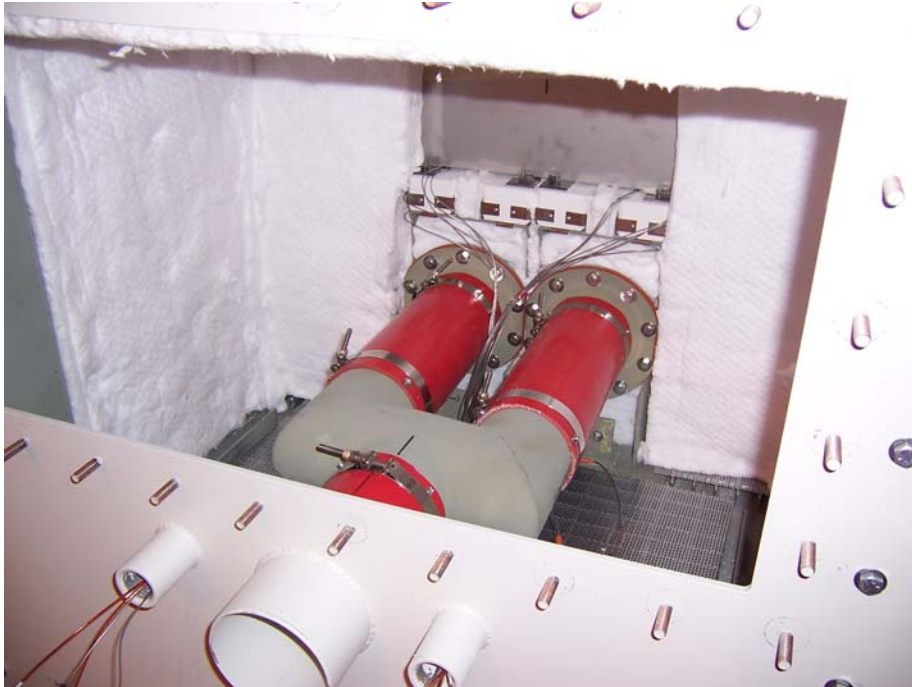
Figure 24 - Air inlet Manifold (as viewed through the container hatch)
