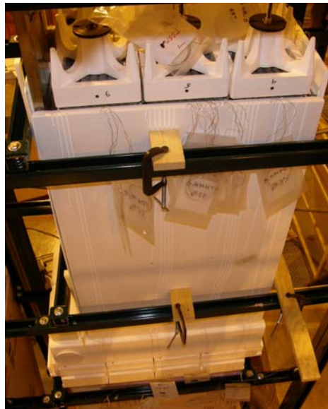
Figure 55 – Stack Assembly: Dielectric Boards, SRZs, and Recirculation Castings
