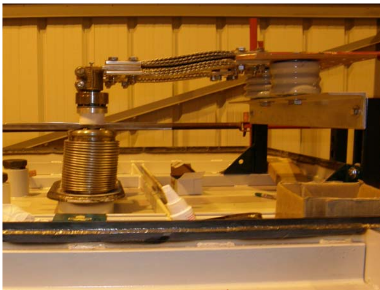
Figure 69 – Power Lead Cables
