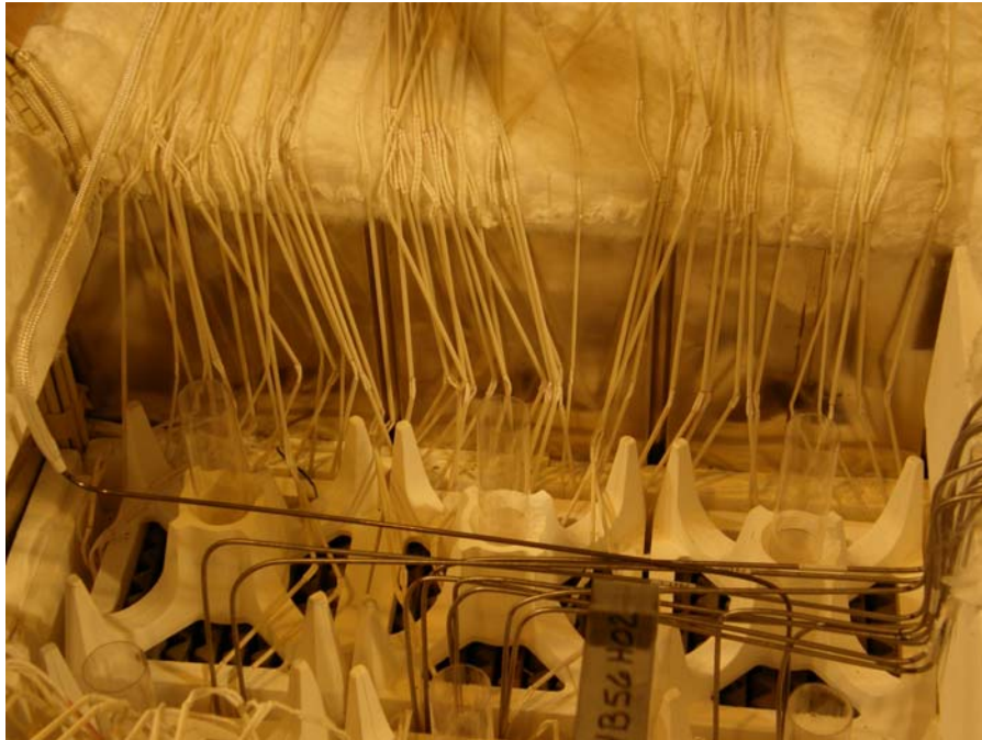
Figure 9 – Instrumentation Leads Crossing over the Stack Liner
