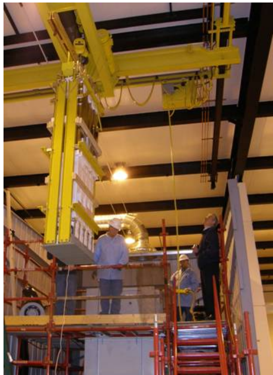
Figure 44 – Stack Test Article Being Installed into Container
