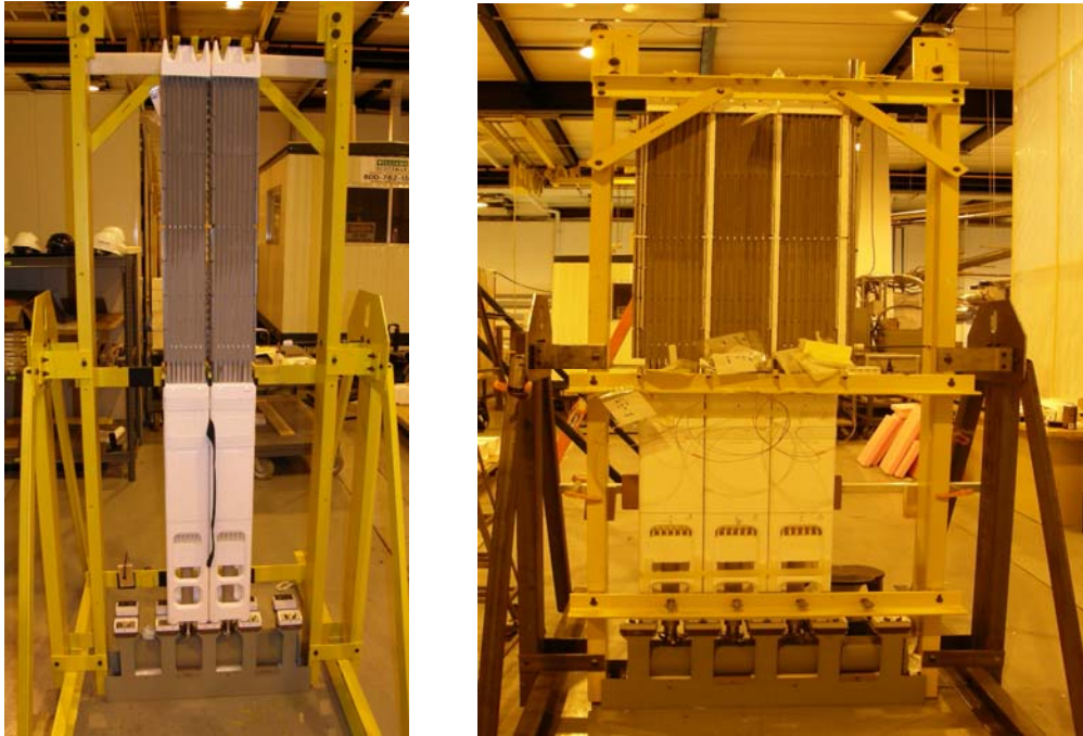
Figure 39 –Bundle Row Assembly Fixture (left, two IBAs; right, three IBAs)
