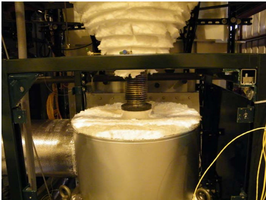
Figure 36 – Prereformer Outlet Bellows (post-test)
