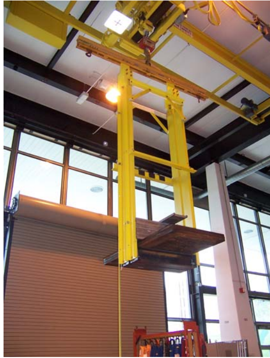
Figure 43 – Stack Lifting Fixture - Proof Load Test
