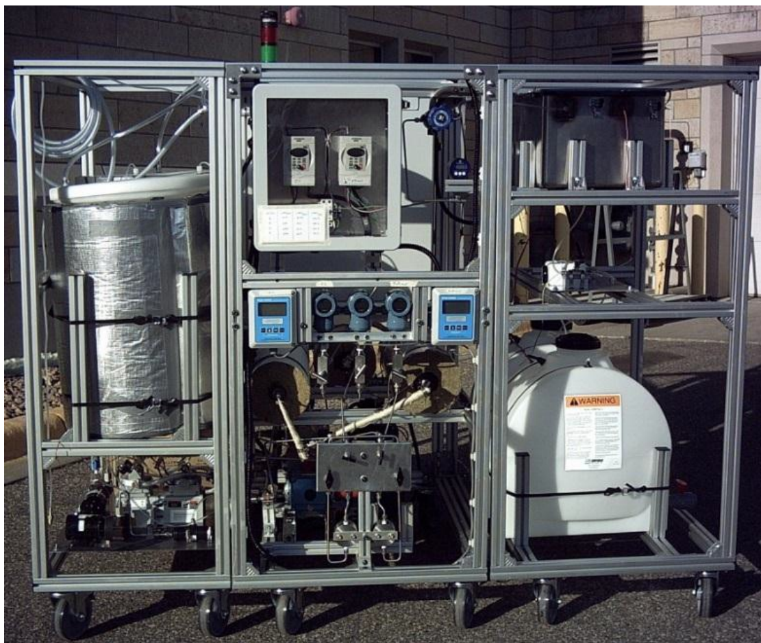
Figure 72. Supercritical Biodiesel Reactor System
