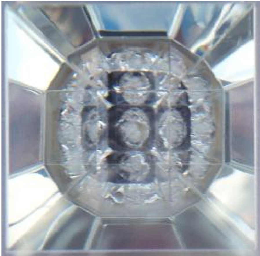
Figure 21. CPV Cell Damage from 500 Suns
