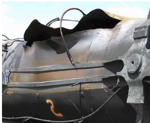
Figure 7-3. Car with Thermal Tear.
