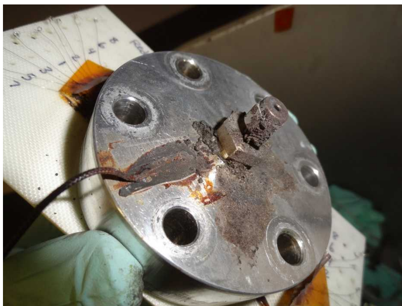
Figure 21. Exp394 post-test residue, showing the top of the vessel with expelled material.
