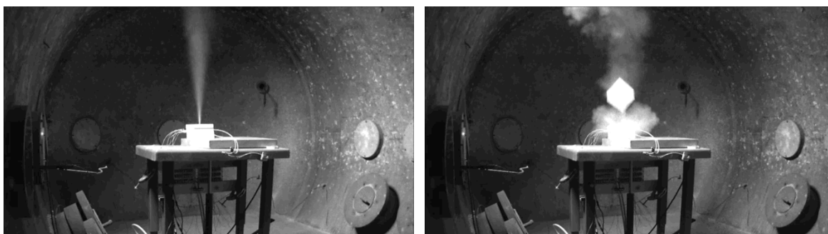
Figure 23. Images from video of Exp395. Left: explosive event at 40.5 minutes. Right: energetic event at 45.1 minutes, showing the top layer of insulation being blown off.
