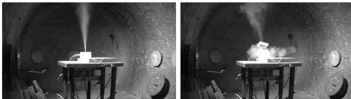
Figure 20. Images from video of Exp394. Left: explosive event at 40.7 minutes. Right: energetic event at 45.9 minutes, showing the top layer of insulation being blown off.
