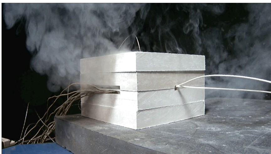
Figure 2. Exp386 video frame showing steam escaping after vessel seal failure.
