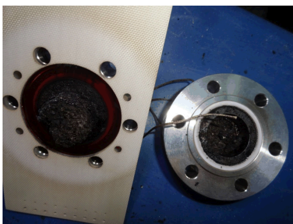
Figure 41. Photo of post-test debris from Exp402.
