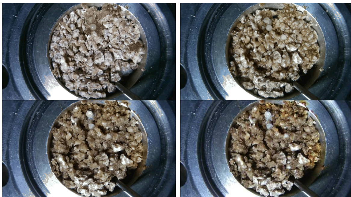
Figure 29. Images from video of Exp397. From left to right, top to bottom: before over-neutralized nitric acid was added, immediately after addition of liquid, 95 minutes into the heating, and 112 min into the test.
