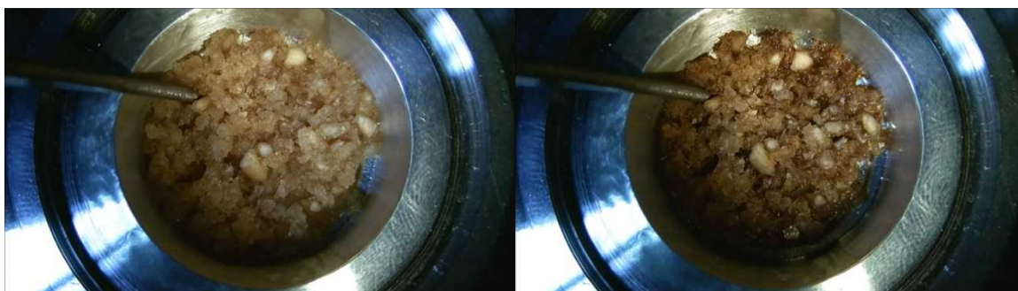
Figure 15. Images taken from video of Exp391. From left to right, top to bottom: before under-neutralized nitric acid was added, immediately after the liquid was added, 92.8 minutes into the test, and 154 minutes into the test.
