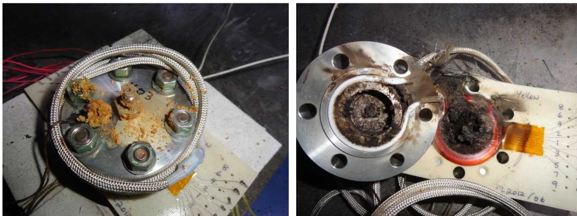
Figure 44. Post-test images from Exp403. The left images shows that a substantial amount of material was expelled through the vent. The right image shows that the O-ring failed.
