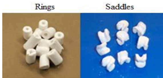
Figure 2 Catalyst Forms Used in Reactive Distillation
