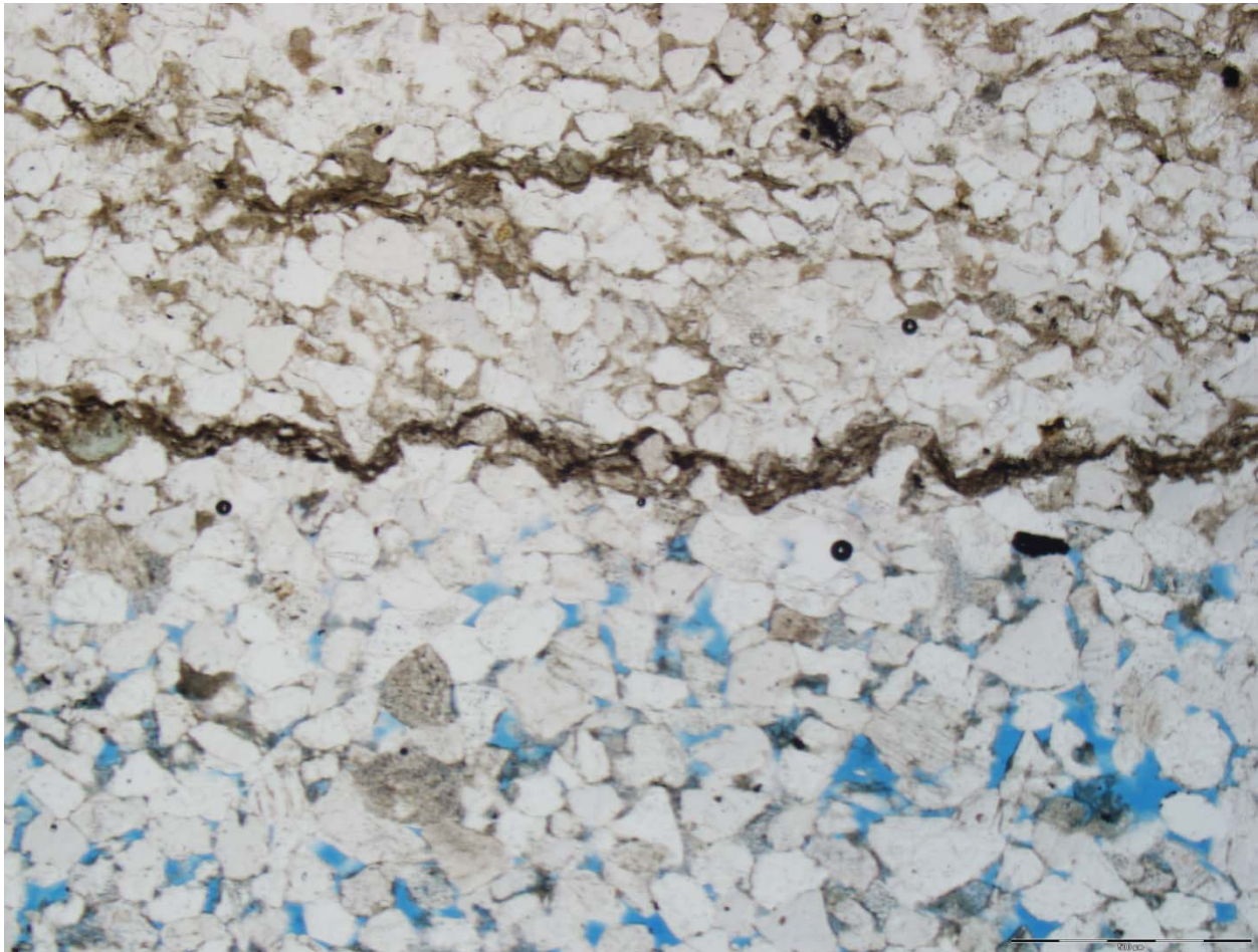
Figure 20 Example from the Griggs #107 at 443 m (1453.4 ft) shows porous laminae alternating with nonporous laminae. Porosity is highlighted by medium-blue stained epoxy. A clay laminae parting separates the nonporous tightly cemented fine-grained sandstone from the porous sandstone.
