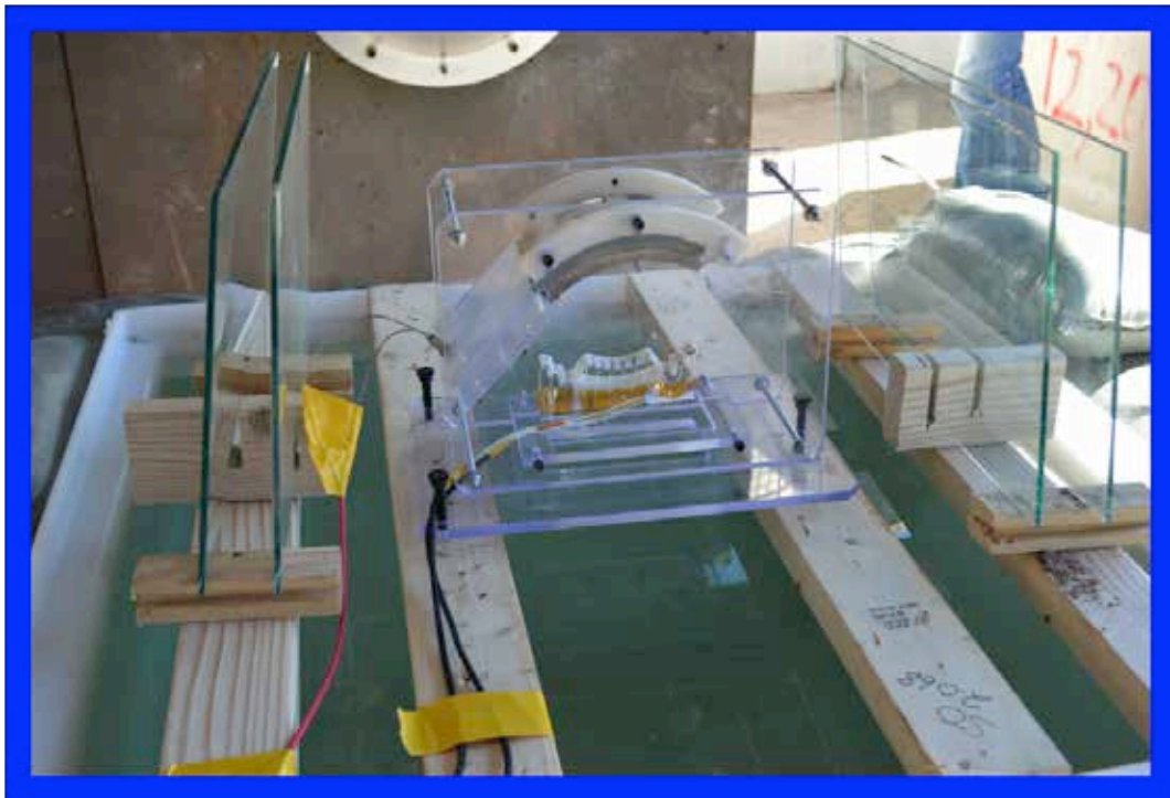
Figure 3. 10cm radius curved Ta sweeping detonation-wave assembly set-up.
