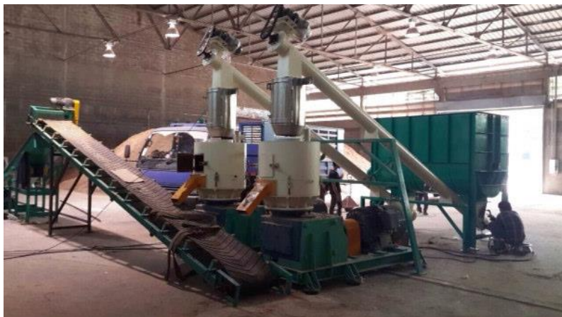
Small pellet mill only setup with a +/- 1,600sf footprint
