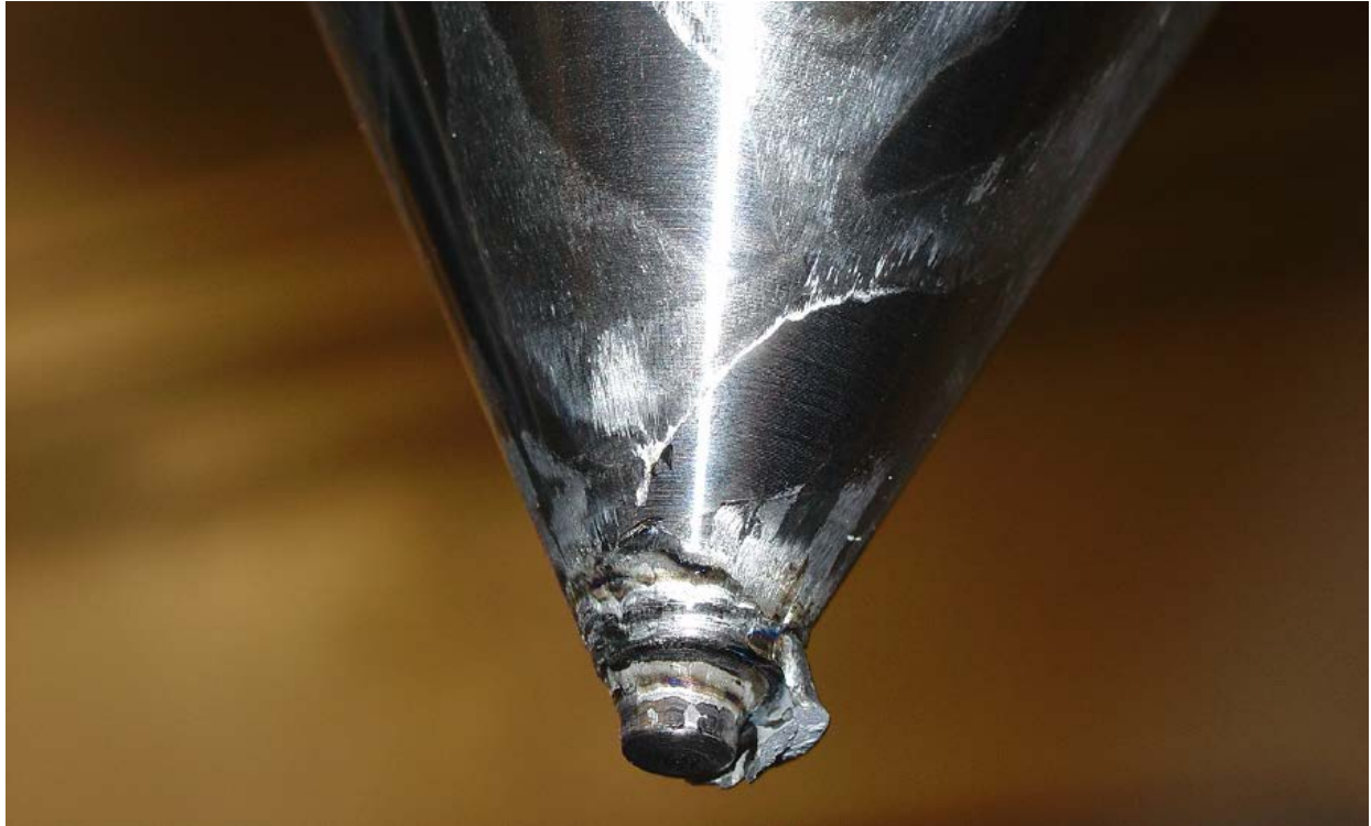
Figure 72. Conical punch following ARP_CP2 test
