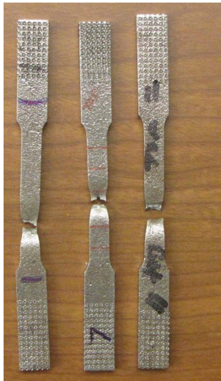
Figure 14. Abrasion-resistant steel tensile samples (post-test)
