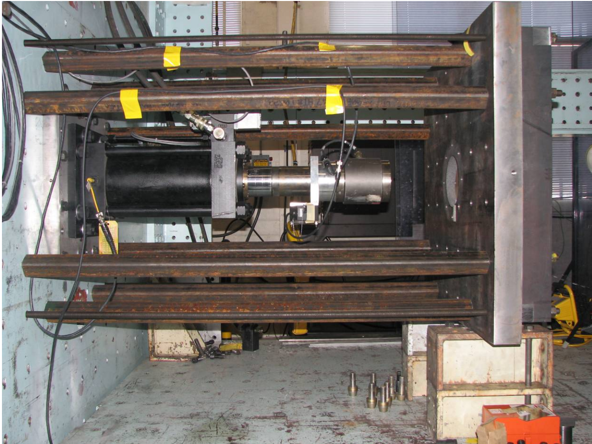
Figure 19. Quasi-static punch plate test setup
