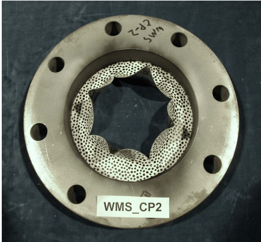
Figure 70. Typical mild steel-conical punch specimen
