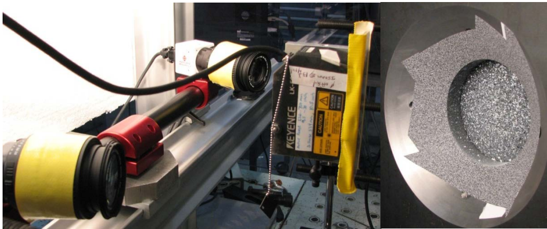
Figure 22. Camera setup and Keyence sensor looking at a speckled sample mounted in the test fixture
