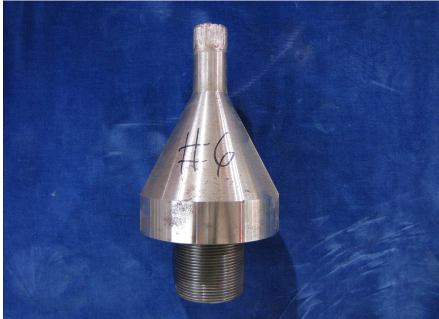
Figure 2. FY07 flat end, 1-inch cylindrical punch
