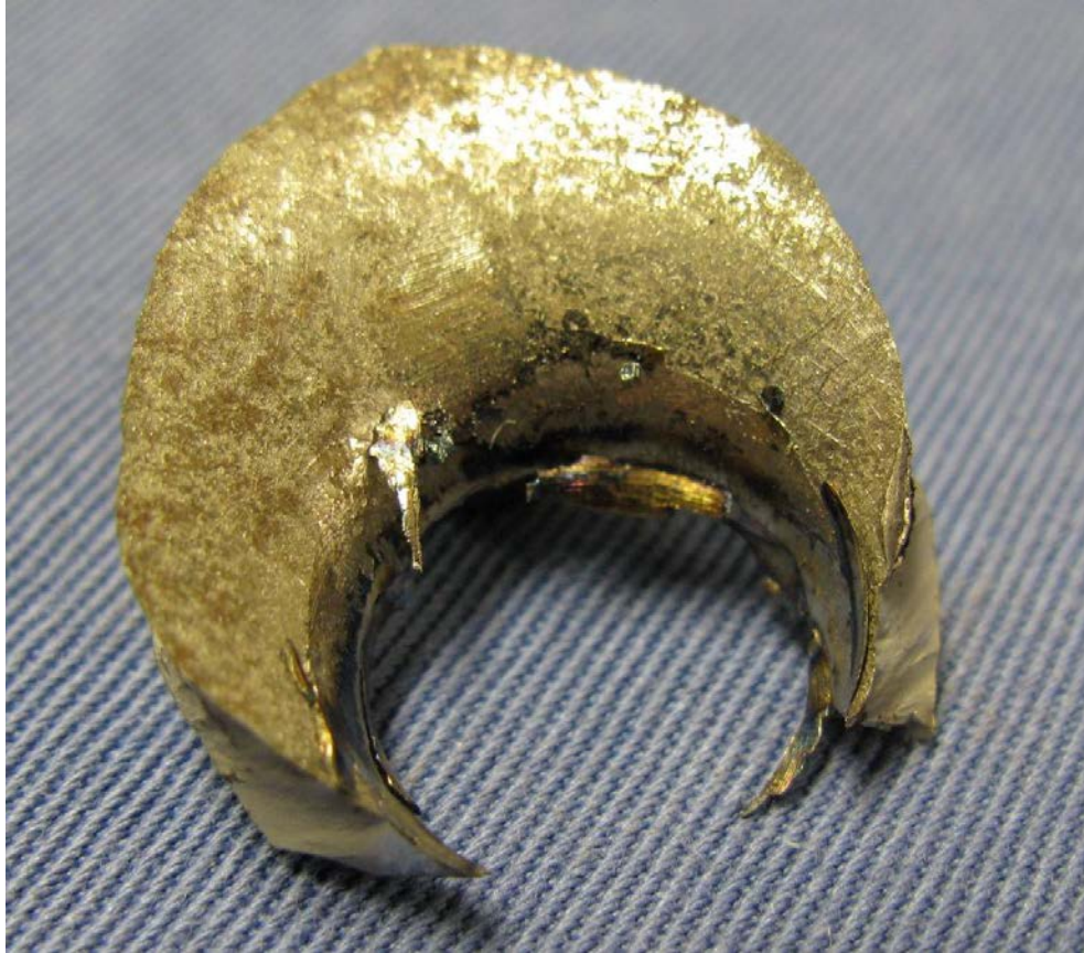
Figure 73. Plate fragment from ARP_CP3 tests showing heat induced discoloration
