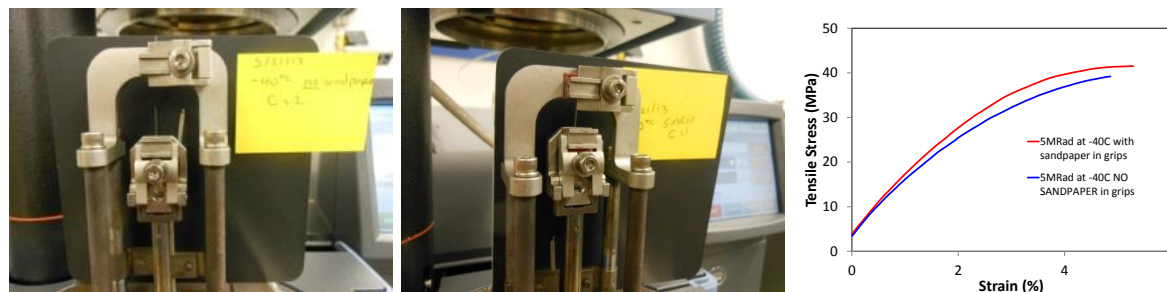
Figure 2-10. Rad exposed fiber modulus measured with and without sandpaper grip.
