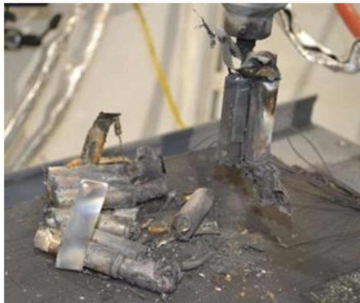
Figure 13. Photograph of the 1S10P battery post-propagation test.
