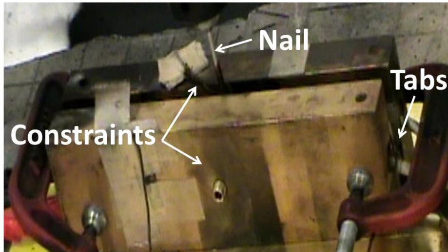
Figure 2. Orientation of nail penetration on single pouch cell.
