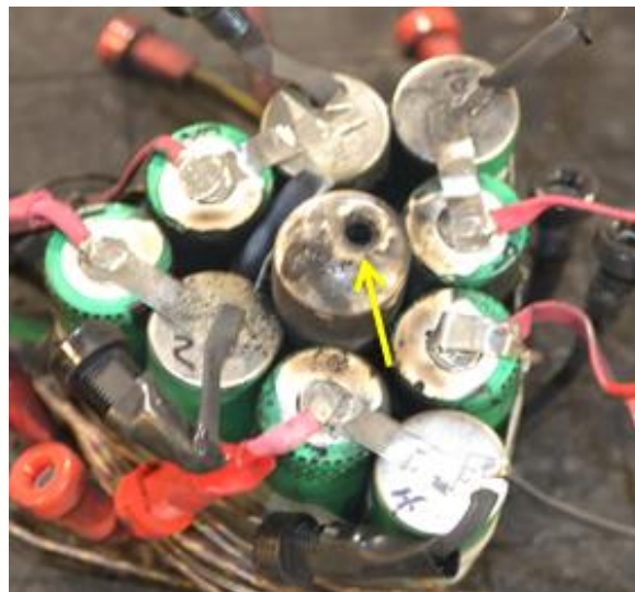
Figure 10. Photograph of the 10S1P battery post-propagation test showing the penetration of Cell 6.
