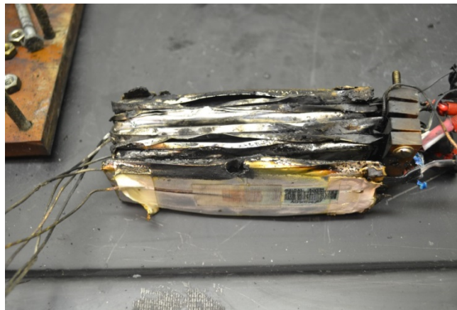
Figure 19. Photograph of the 5S1P battery post-propagation test initiated at Cell 1.
