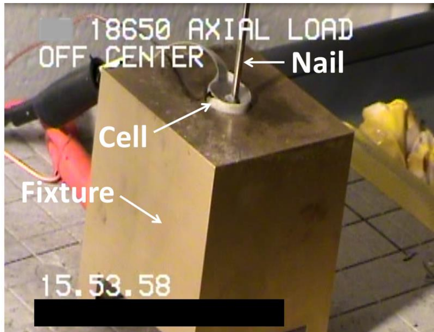
Figure 1. Orientation of nail penetration on single cylindrical 18650 cell.
