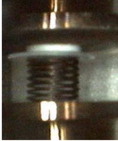
Figure 6.2. Wave spring validation test setup within the ARES 2 rheometer. The wave spring, sapphire plate, and separator pellet are visible in ascending order between the stainless steel platens.
